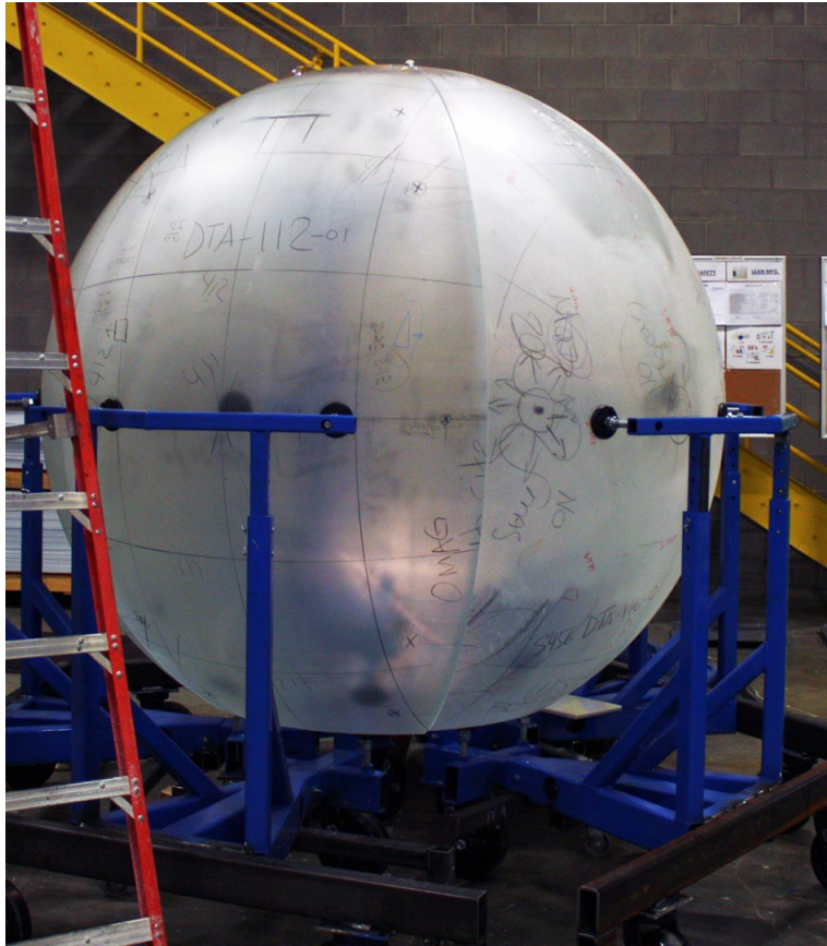
Figure 2.5: Photograph of the dry fit of the 5 acrylic gores that compose the main AV. Photo credit RPT.
