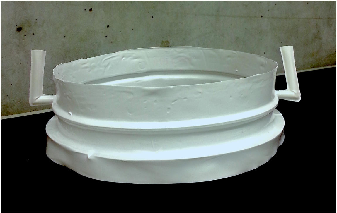
Figure 3.5: Fully formed polyethylene dam pre-installation.
