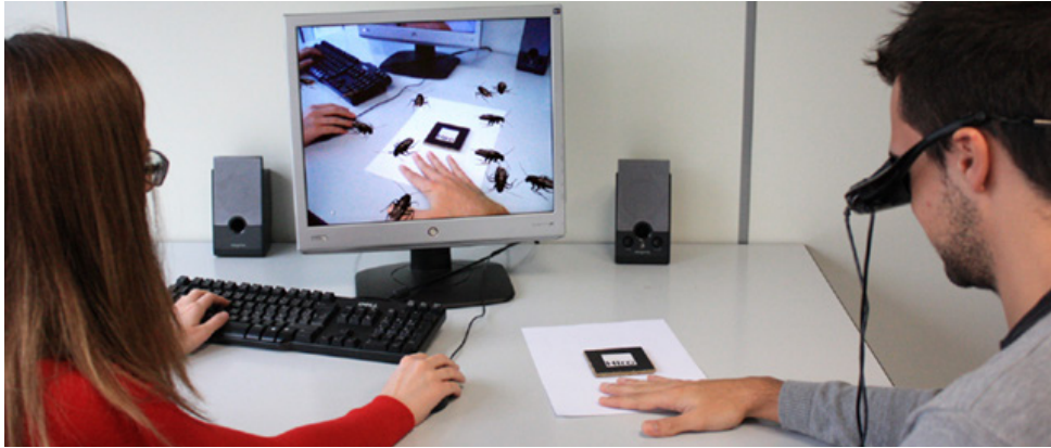
Figure 6: The black marker on the paper is the VMARS (Visible Marker-tracking Augmented Reality System). Copyright. Labpsitec. Universitat Jaume I. Spain.
