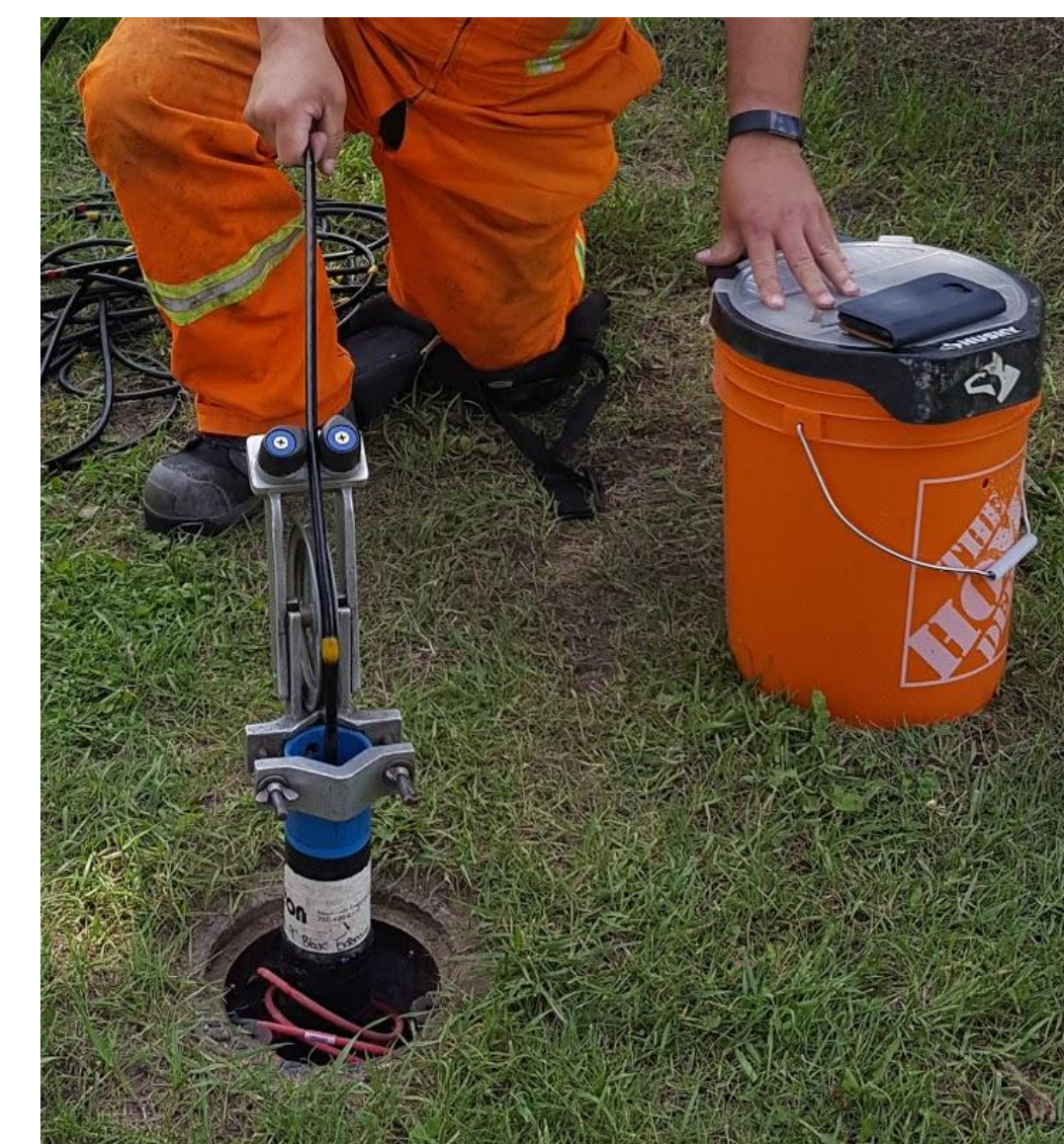
Figure 3.0 A technologist taking slope inclinometer (SI) measurements.
