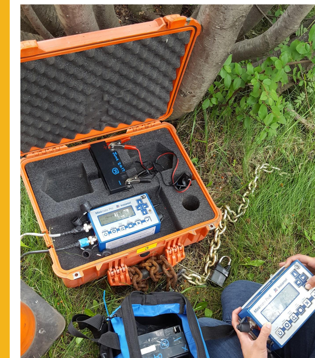
Figure 5.0 A technologist monitoring vibrations near a construction site.
