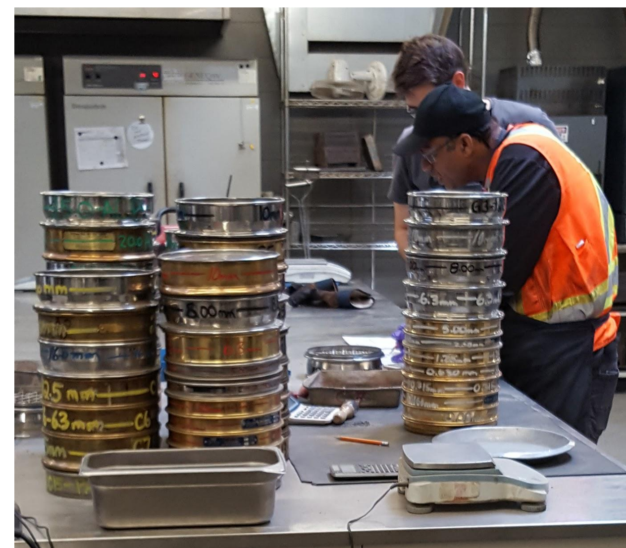
Figure 2.0 A technologist in the asphalt lab sieving and weighing aggregate.
