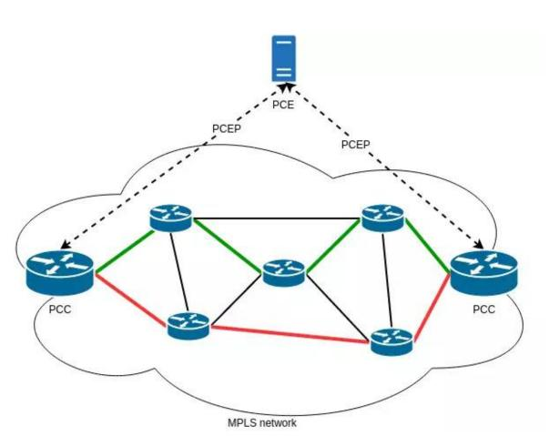
*Fig3.3: PCE-based architecture*
