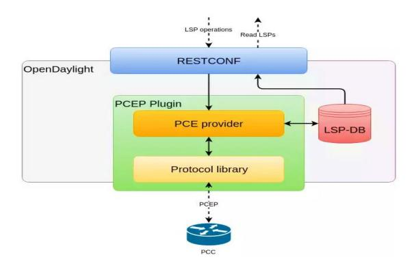
Fig 2.2 : Opendaylight OpenFlow PCEP Plugin
