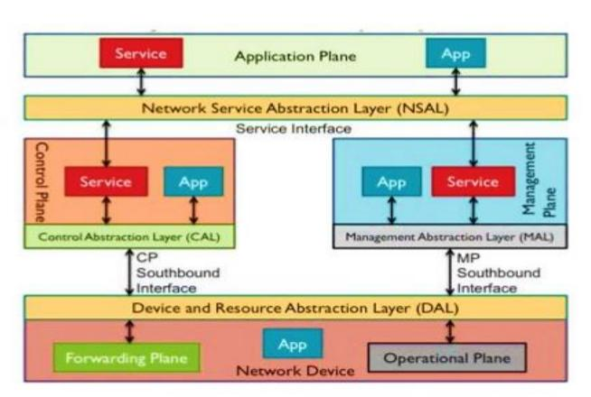
Fig 1.2: SDN Layer Architecture
