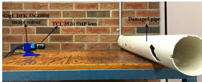
Figure 3.4: Dataset acquisition setup.
