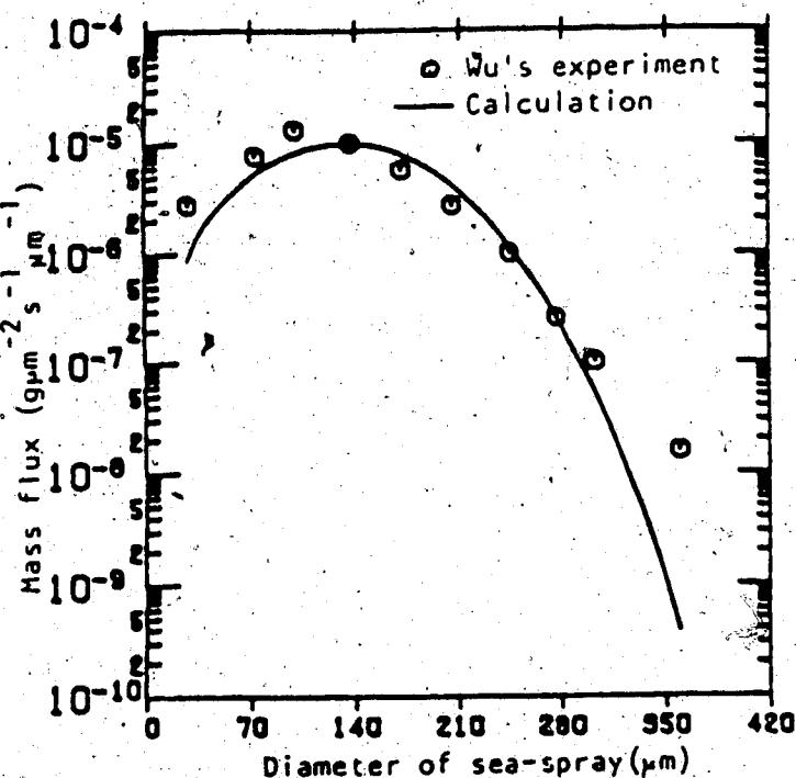
Fig. 8 Mass flux of sea-spray at the ocean surface.
