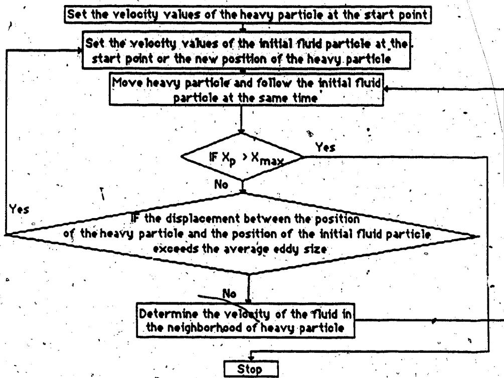
Fig.3. Flow chart of heavy particle trajectory model
