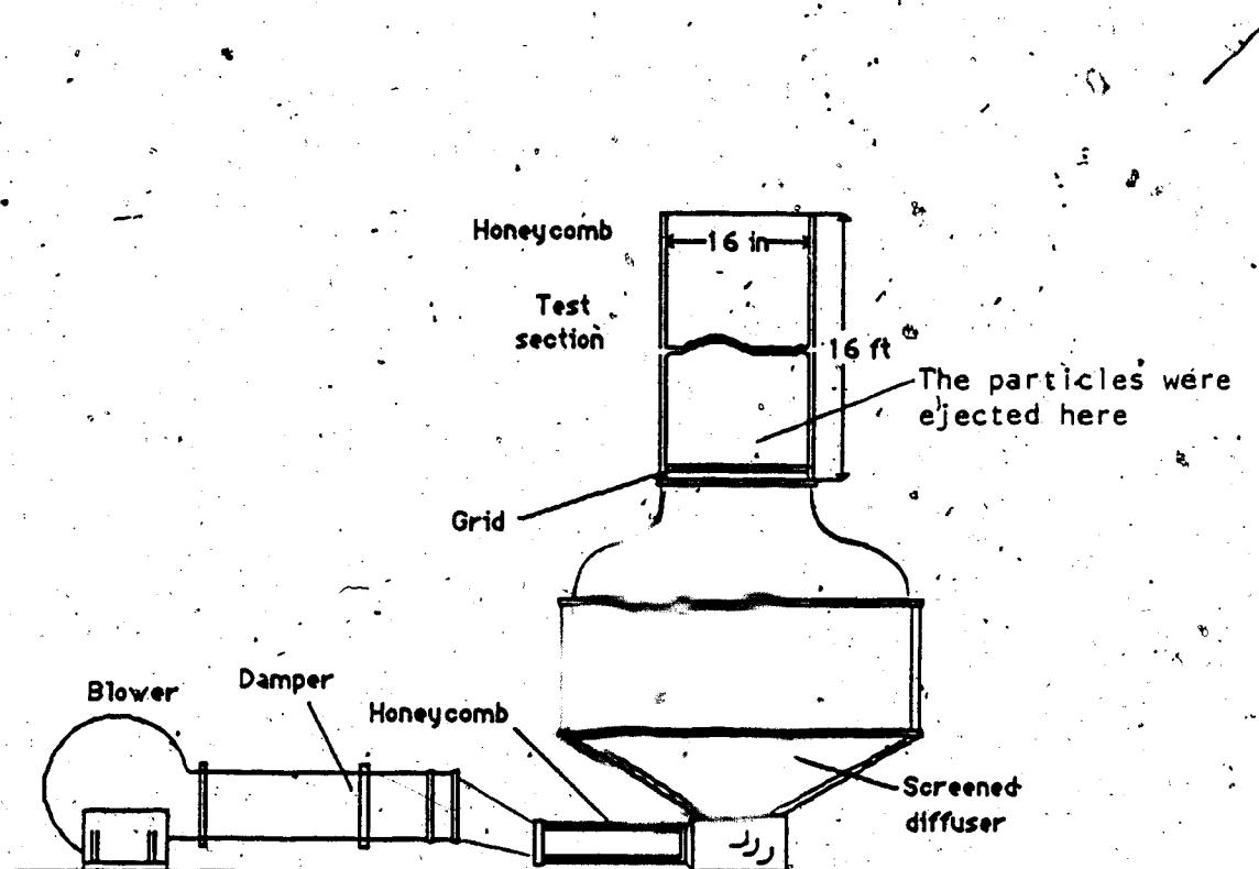
Fig.4. The wind tunnel of Snyder and Lumley's experiment
