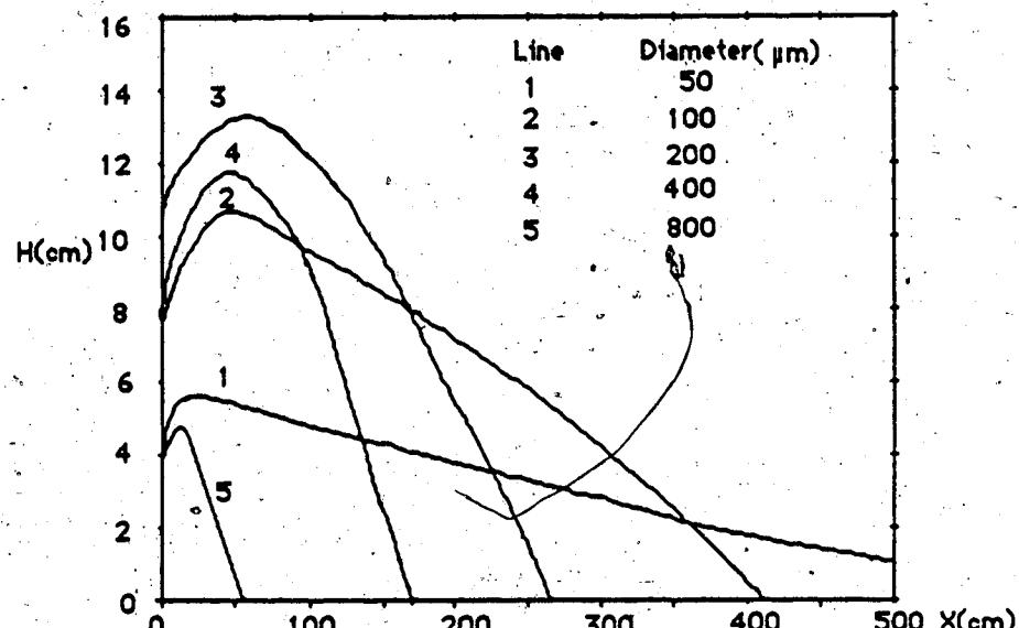
Fig.10 Droplet trajectories in a laminar flow.
