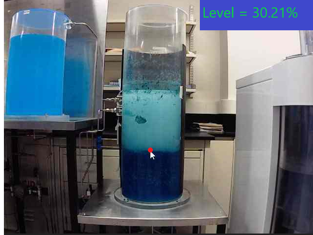
Figure 3.6: Labelling of image using mouse-click at the location of the interface.
