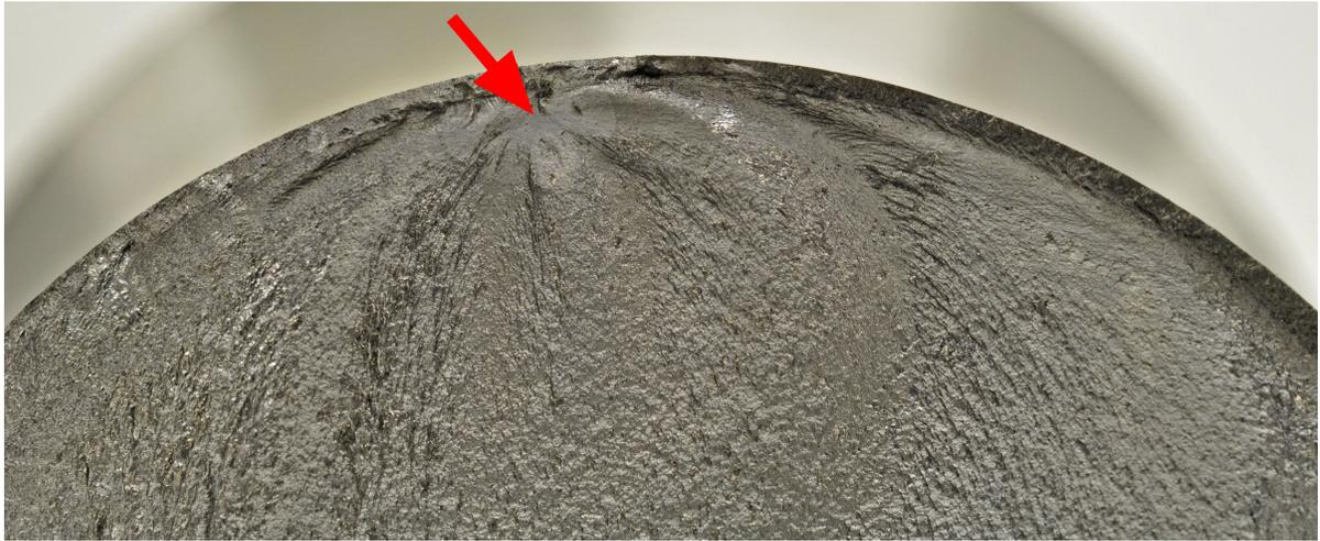
**Figure 7.36:** C-30 coupon fracture initiation at a non metallic inclusion in the HAZ
