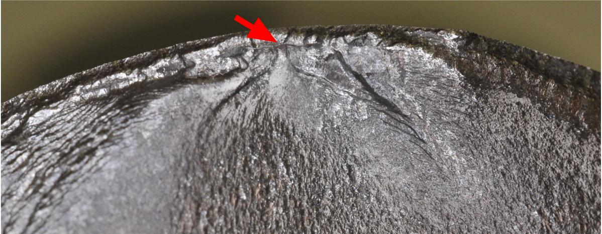
**Figure 7.39:** D-NO coupon fracture initiation at a fusion line discontinuity
