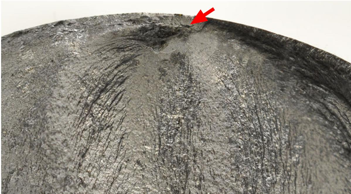
**Figure 7.31:** B-NO coupon fracture initiation at a fusion line oxide
