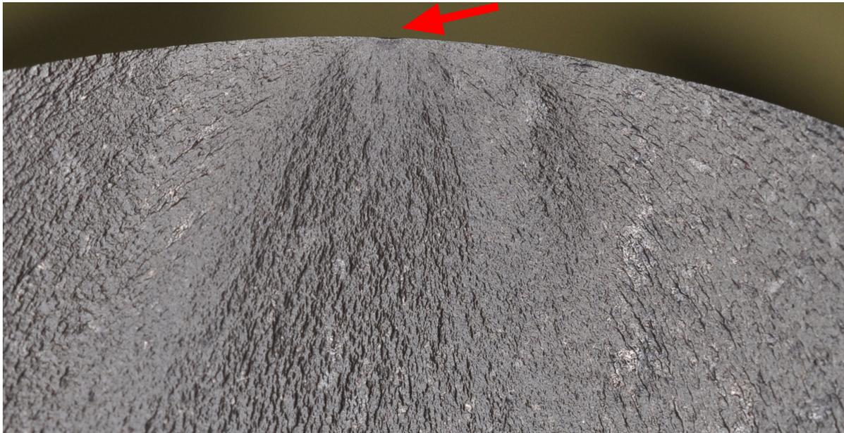
**Figure 7.25:** A-CO coupon showing fracture initiation at a "dent" in the surface
