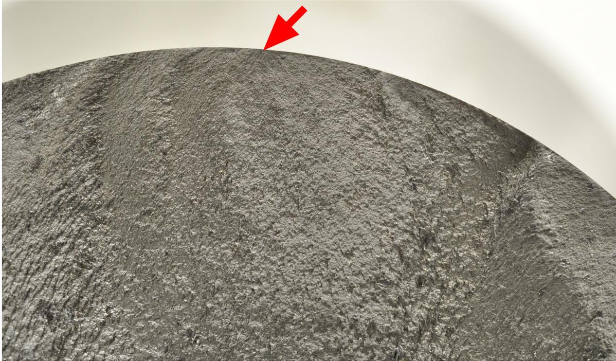
**Figure 7.42:** E-CO coupon fracture initiation at the surface
