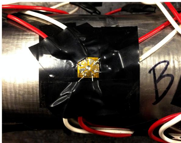
**Figure 8.62:** RS-30 strain gauge rosette installation
