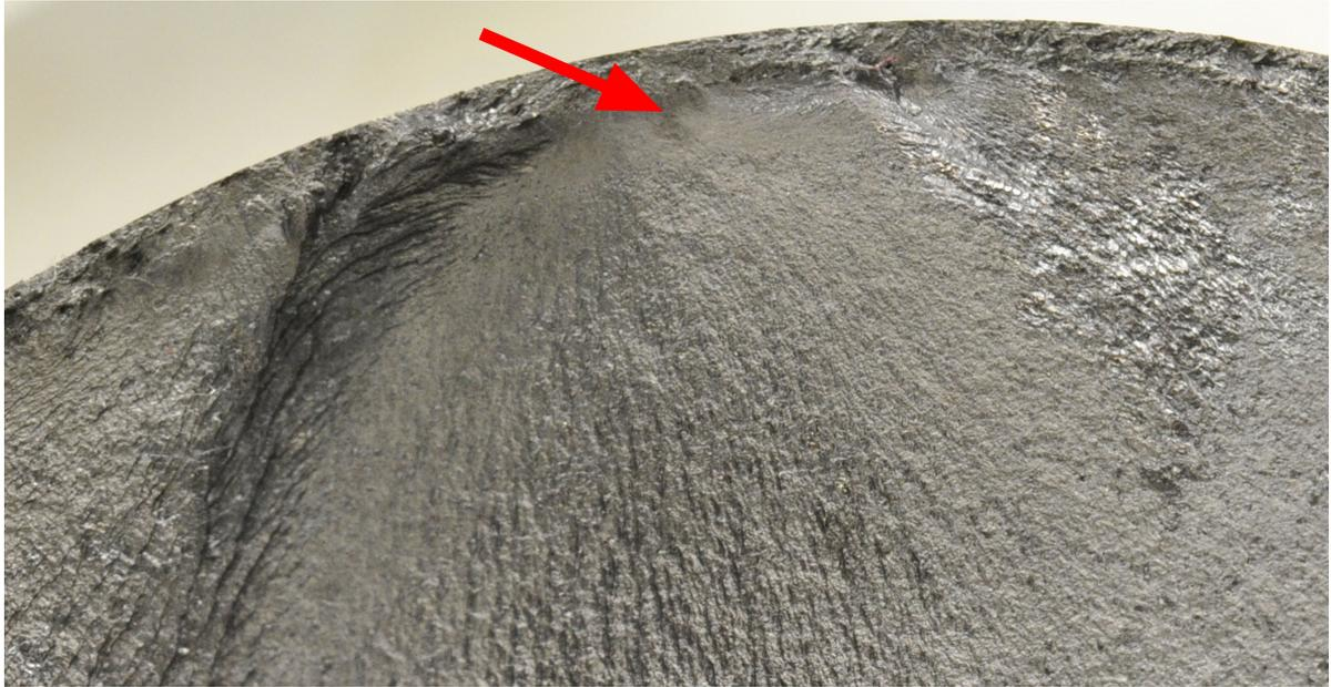
**Figure 7.50:** Location 1 of the F-30 fracture shown in Figure 8.49. Initiation occurred at a non metallic inclusion in the HAZ
