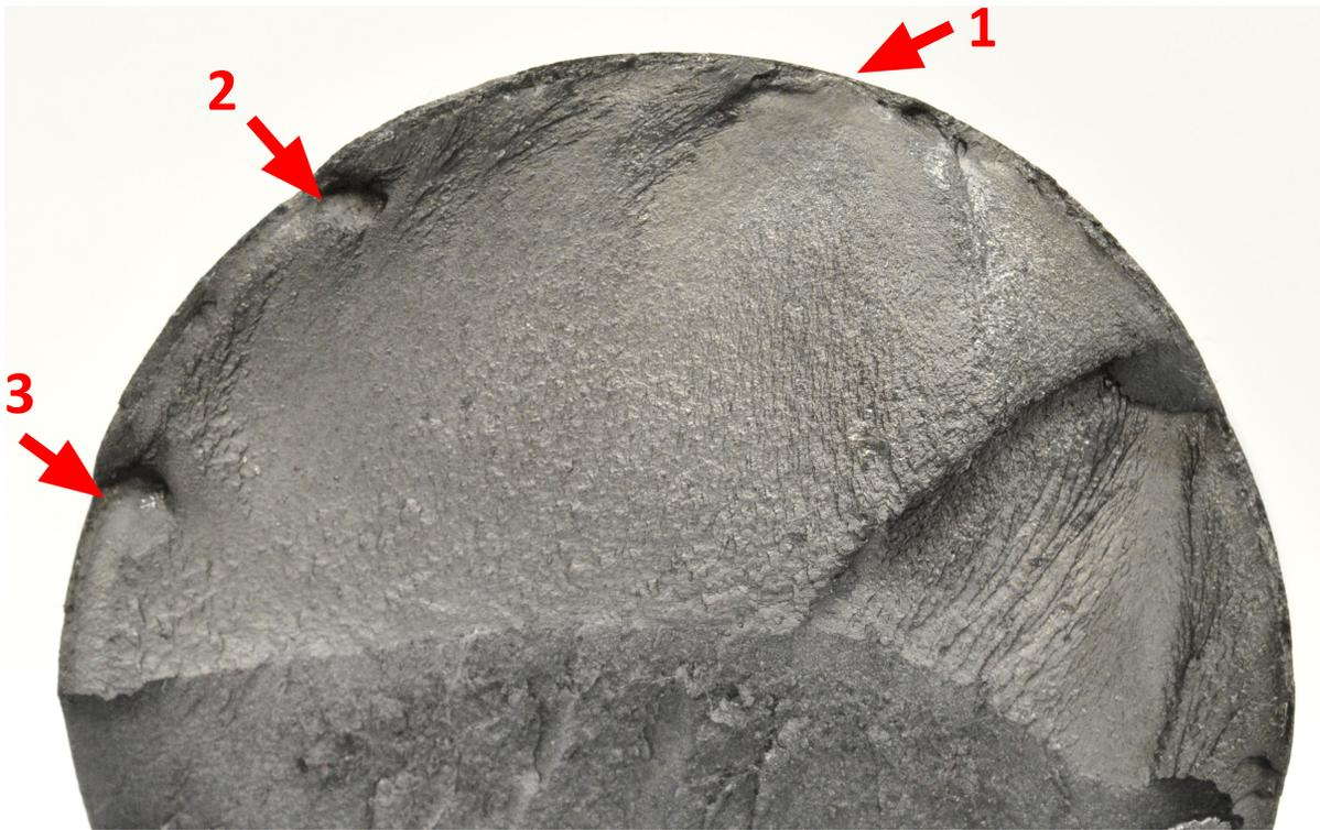
**Figure 7.49:** F-30 coupon showing multiple fracture initiation locations. The fracture initiated at location 1 dominated failure
