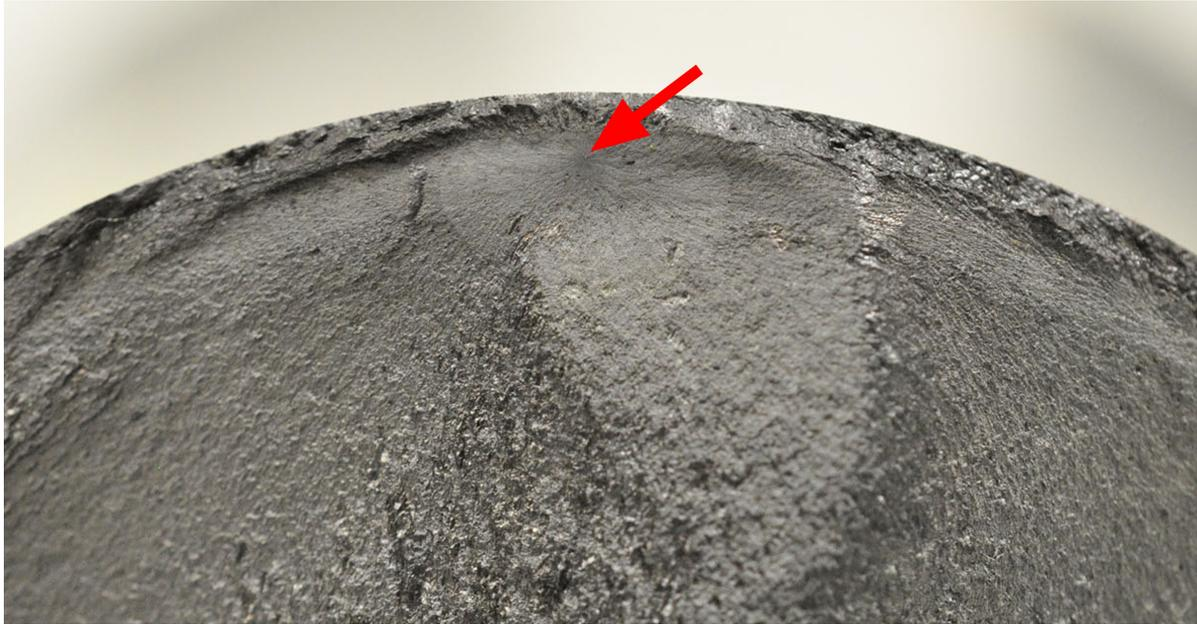
**Figure 7.33:** B-60 coupon fracture initiation at a non metallic inclusion located in the HAZ
