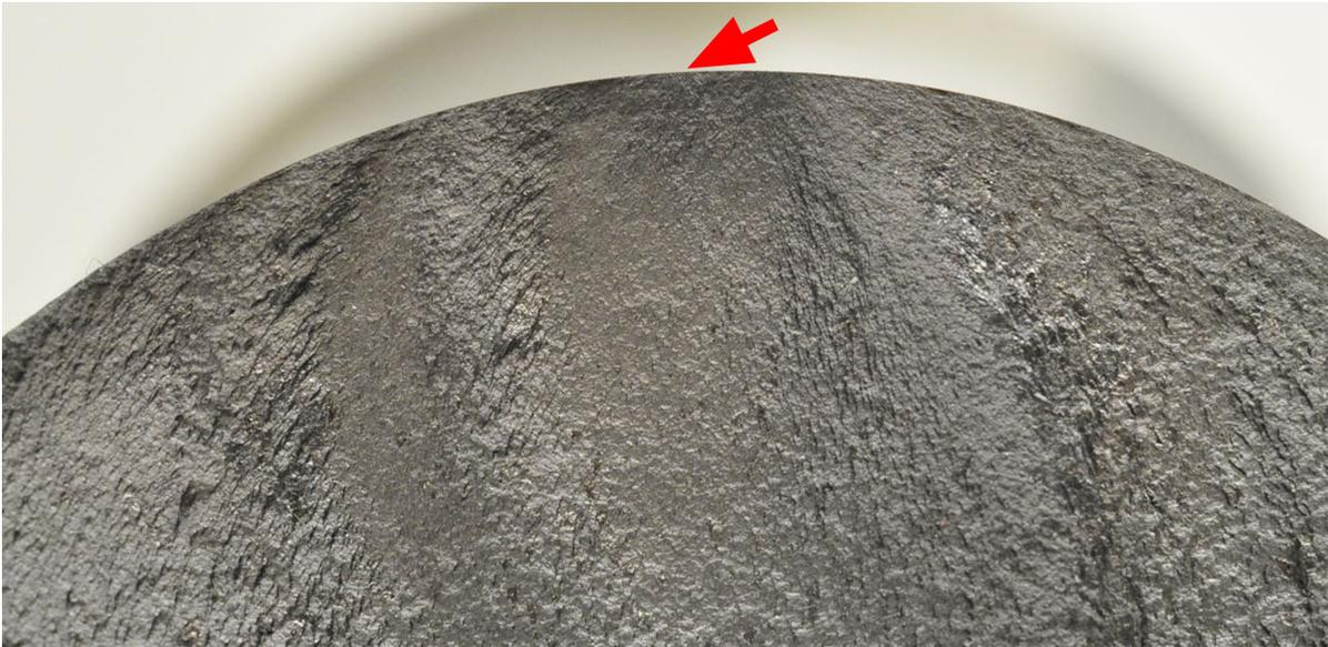
**Figure 7.30:** B-CO coupon fracture initiation at the surface
