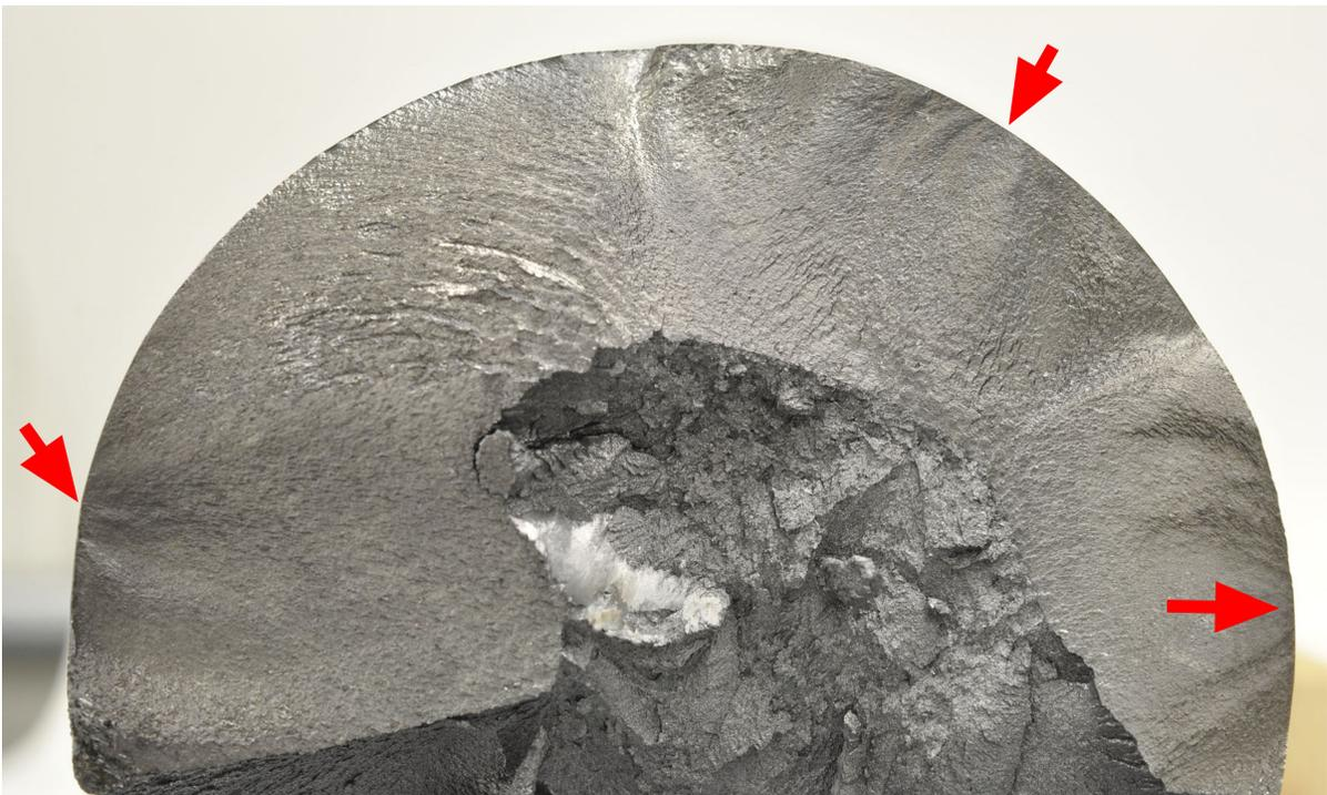
**Figure 7.38:** D-CO coupon fracture initiation at multiple locations on the surface
