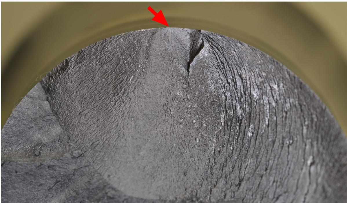
**Figure 7.47:** F-CO coupon surface initiation of the upper fracture shown in Figure 8.45.
