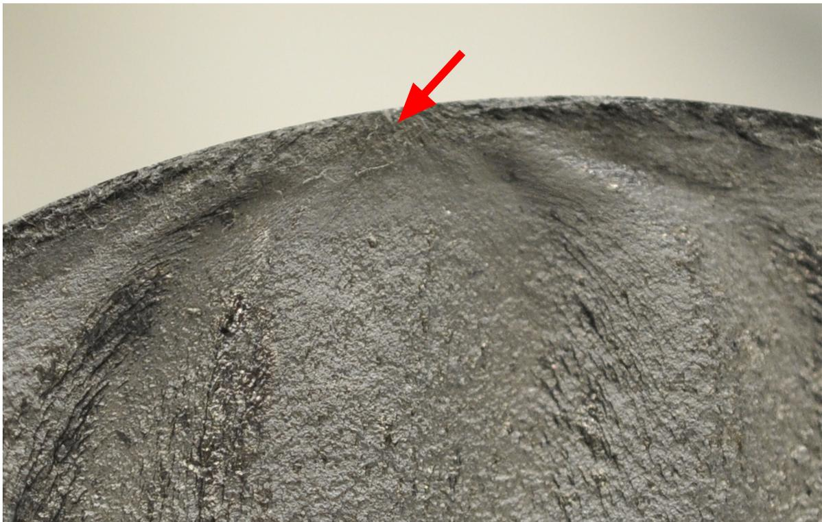
**Figure 7.29:** A-60 fracture initiation at a circular entrapped oxide in the overlay region
