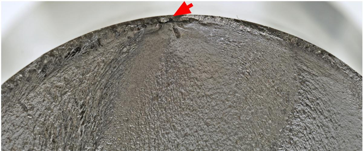
**Figure 7.37:** C-60 coupon fracture initiation at a fusion line discontinuity
