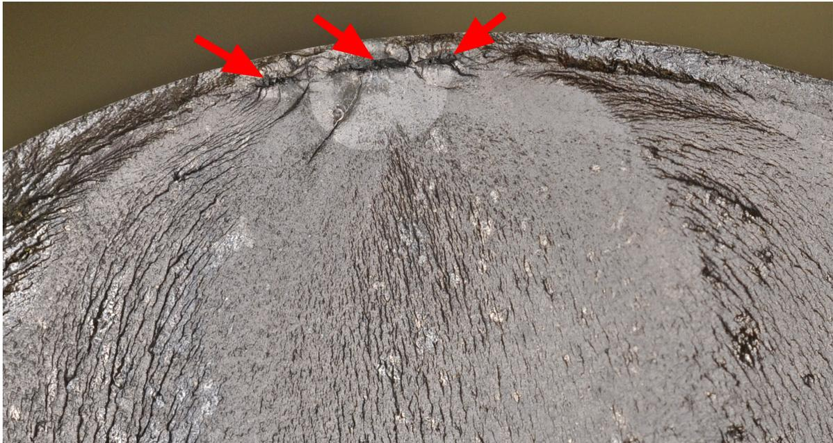
**Figure 7.28:** A-30 fracture initiation at an multiple adjacent entrapped oxides located at the fusion line
