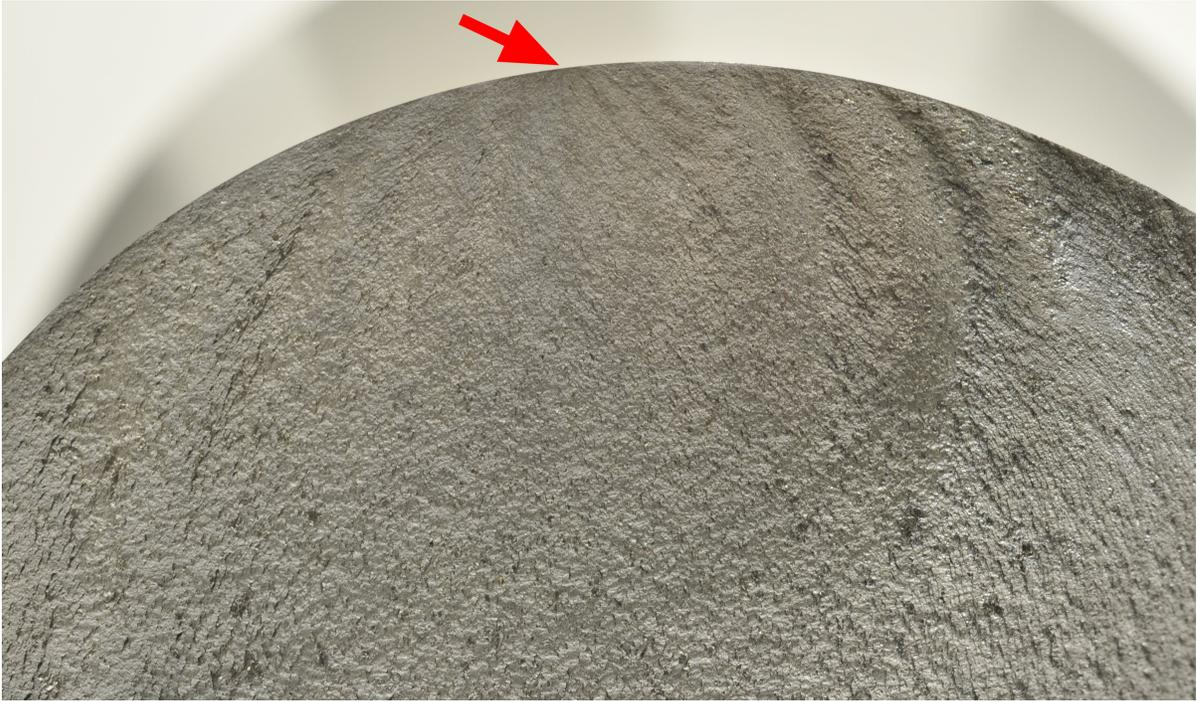
**Figure 7.34:** C-CO coupon fracture initiation at the surface
