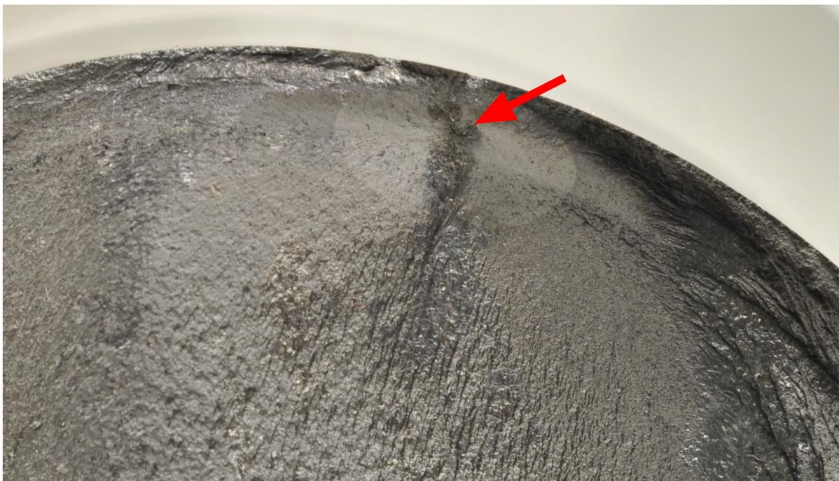
**Figure 7.43:** E-30 coupon fracture initiation at a non metallic inclusion located in the HAZ
