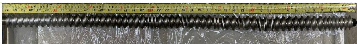
Fig. 1.2 Screw profile developed for production of TVP rotating clockwise with the protein melt flowing from the feeding zone (left) to the die end (right).
