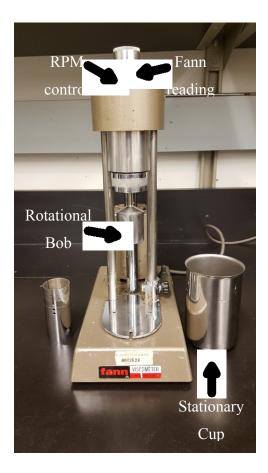
Figure 2-3 Fann viscometer device
