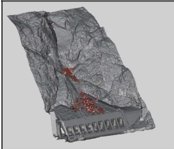
Fig. 2: 1000 fragment rockfall simulation result using discrete and variable fragment shapes. Total volume is 100m 3 . Modified after Sala et al. (2019).
