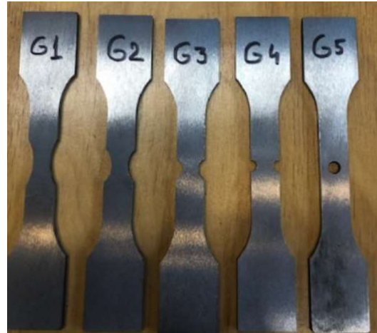
Figure 7. Five damage geometries to measure crack initiation response of TC128B
