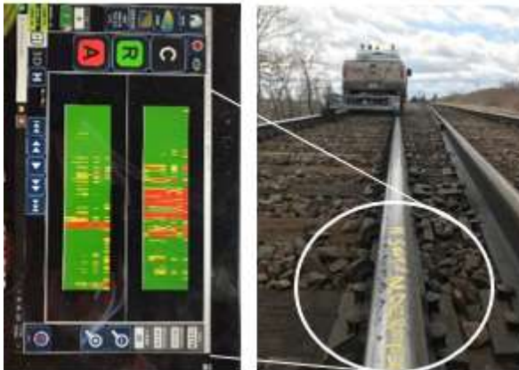
Figure 4. Rail surface quantification using Electromagnetic Field Inspection (EMFI) probes from the rail running surface of a North American Class I railway.
