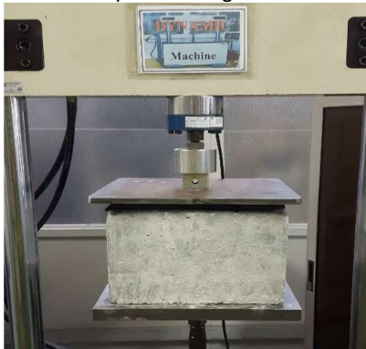
Figure 2. A sample of dynamic bedding modulus test on a specimen of DT-USPs over a concrete block.
