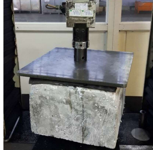
Figure 1. Static bedding module test, a sample of DT-USPs over concrete block under loading jack.
