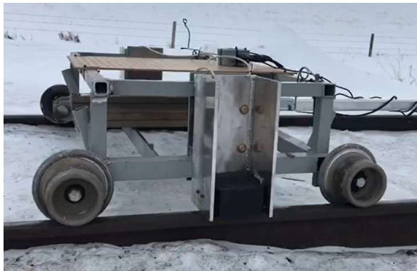
Figure 9. Trolley carrying the Electromagnetic Field Inspection (EMFI) sensors (one per rail) used to perform the rail surface quantification to determine levels of Rolling Contact Fatigue (RCF).
