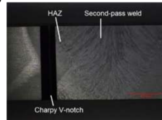
(b) Charpy V-notch at HAZ of the second-pass weld
