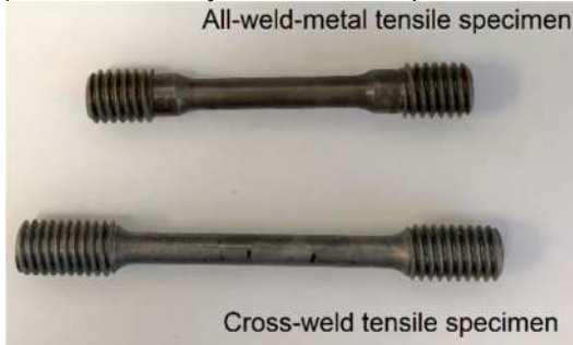
(b) All-weld and cross-weld tensile specimens Figure 2. TC128B tensile specimens.
