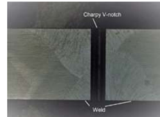
(a) Charpy V-notch at the weld
