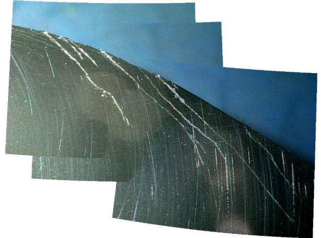
Figure 7. Microscope photography of a polished rail sample shows crack propagation from the checking to the rail head
