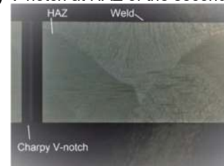
(c) Charpy V-notch at HAZ of the first-pass weld
