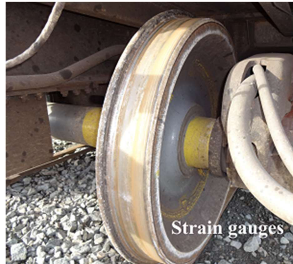
Figure 1. Photograph of an IWS installed on the Gondola railcar. Wheatstone bridge strain gauges and connectors covered in yellow epoxy coating are visible in the photograph (photo credit Hendry 2014).
