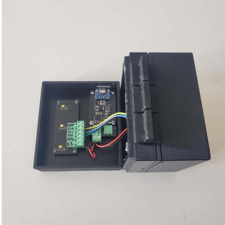
Figure 2.10. Physical assembled bottom layer of the 3-well sensor with a three LED lighting board installed
