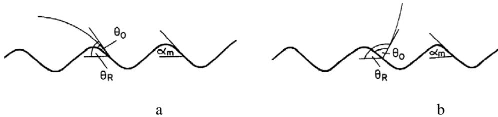
*Figure 3-23. The effect of roughness on the observed contact angles (a). wetting drop resting on a rough surface (b). non-wetting drop resting on a rough surface.<sup>67</sup>*
