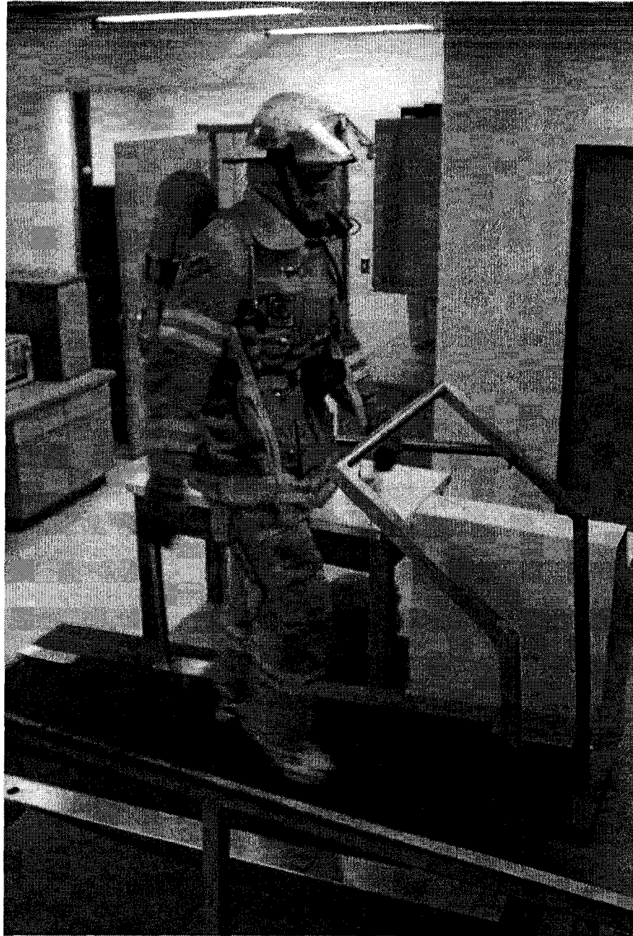
Figure C-5. Experimental set-up for GXT condition in Project Three (Chapter 5). Subjects wore typical exercise clothing (Figure B-1) and full personal protective ensemble while breathing through a Hans Rudolph full-face mask.
