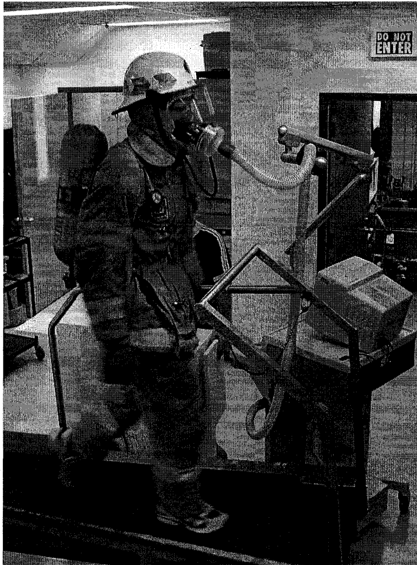
Figure C-2. Experimental set-up for the GXT PPE in Project Two (Chapter 4). Subjects wore typical exercise clothing (Figure B-1) and full personal protective ensemble while breathing through an SCBA. Expired gases were collected via Plexiglass cone interfaced with the SCBA.
