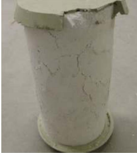
Figure 6.3 Failure of Cylinder for Fibre-reinforced Hydraulic Lime Mortar under Compression
