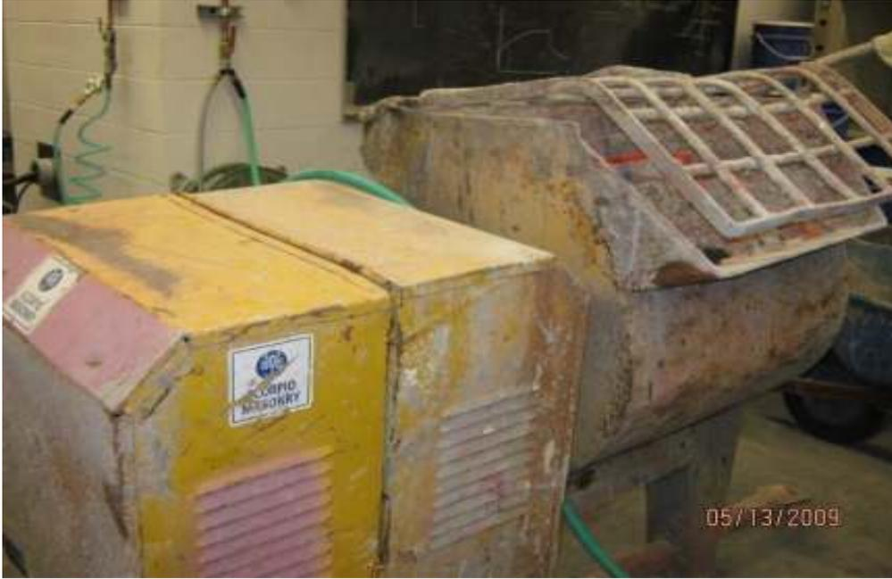
Figure 3.4 Mortar Mixture Machine
