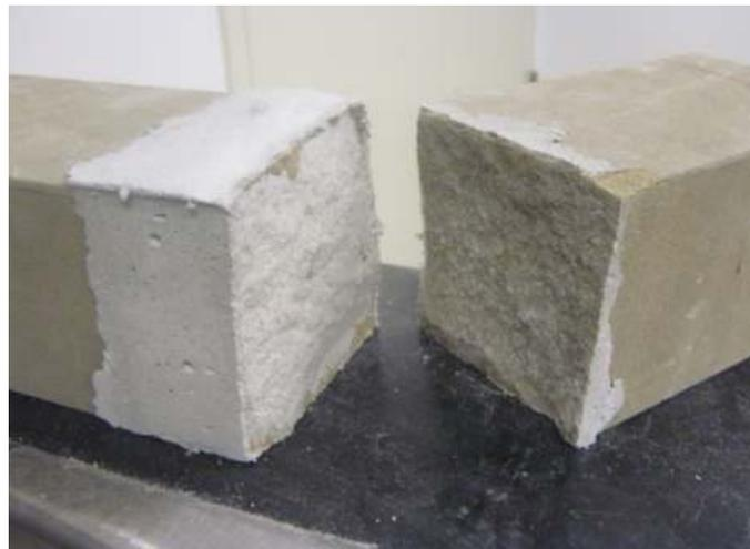
Figure 5.6 Failure of Masonry Unit for Plain Type S Mortar under Flexure. Note Failure Plane at the Stone-mortar Interface.
