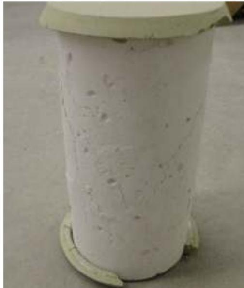
Figure 6.2 Failure of Cylinder for Plain Hydraulic Lime Mortar under Compression
