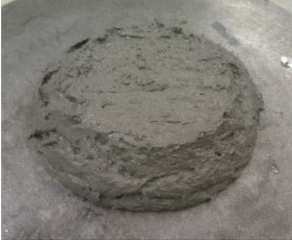
Figure 7.3 Flow Test with Fibre-reinforced Mortar as per ASTM 1437
