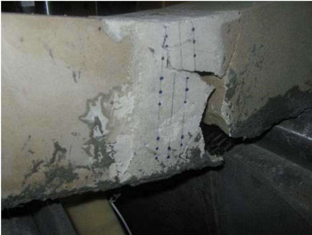
Figure 7.8 Mode of Failure of Composite Sandstone/CTRM Specimen Unit-R-0
