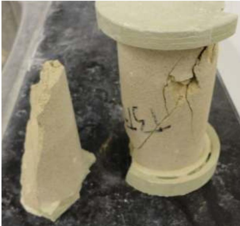
Figure 4.3 Failure of a Sandstone Cylinder under Compression
