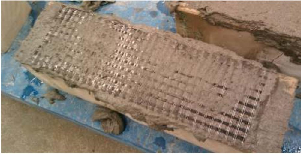
Figure 7.5 Masonry units under Repair using CTRM
