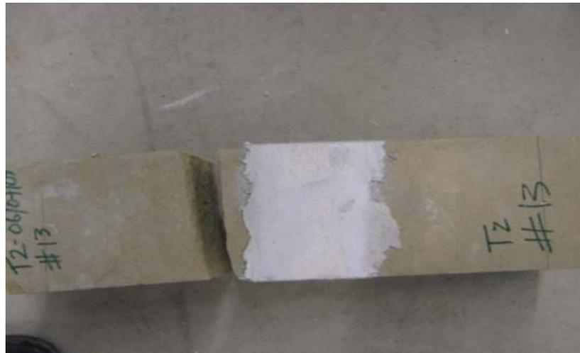
Figure 5.7 Failure of Masonry Unit for Fibre-reinforced Type S Mortar under Flexure. Note Failure Plane passes through the Stone Block.
