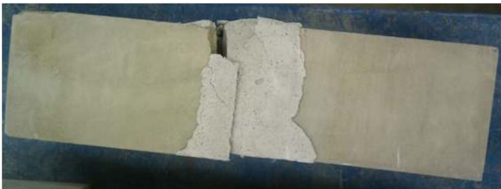
Figure 7.4 Example of Failed Masonry Units after Testing as described in Section 3.4.1.2 and Section 3.4.2. The broken Unit was re-assembled prior to Strengthening.
