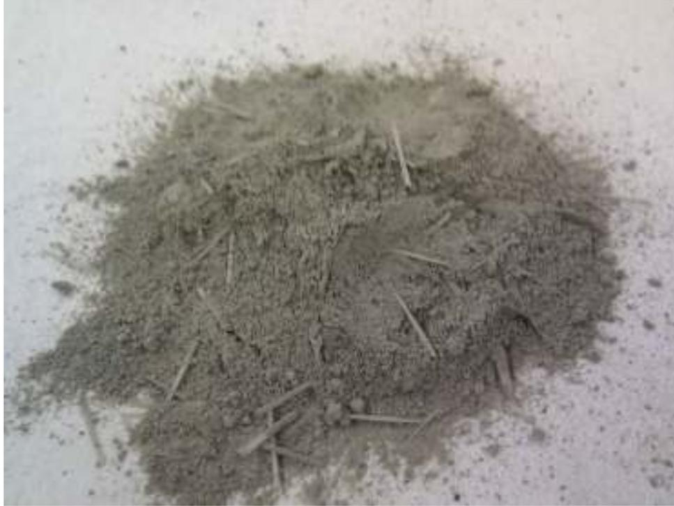
Figure 7.1 Premixed Fibre-reinforced Mortar M25 used to apply the CTRM
