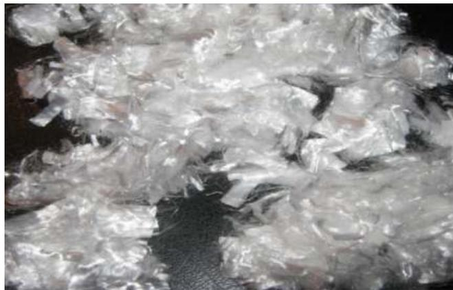
Figure 3.3 Polypropylene Microfibres used in this Study
