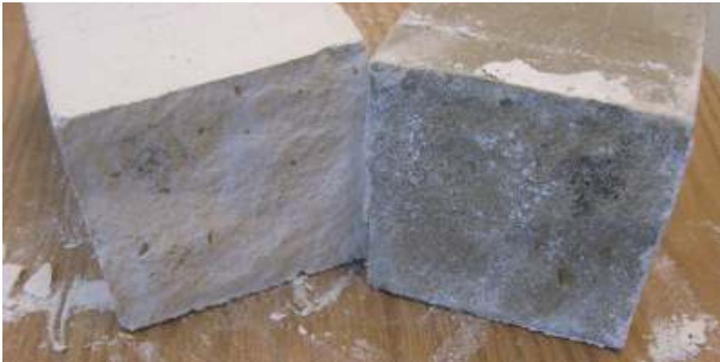
Figure 6.11 Failure of Masonry Unit at the Stone-Mortar Interface
