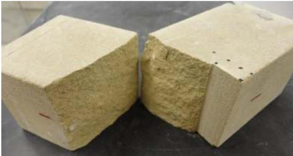
Figure 4.7 Failure of a Sandstone Prism under Flexure
