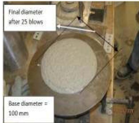
Figure 3.5 Workability of Mortar Mixes as Determined by a Flow Table
