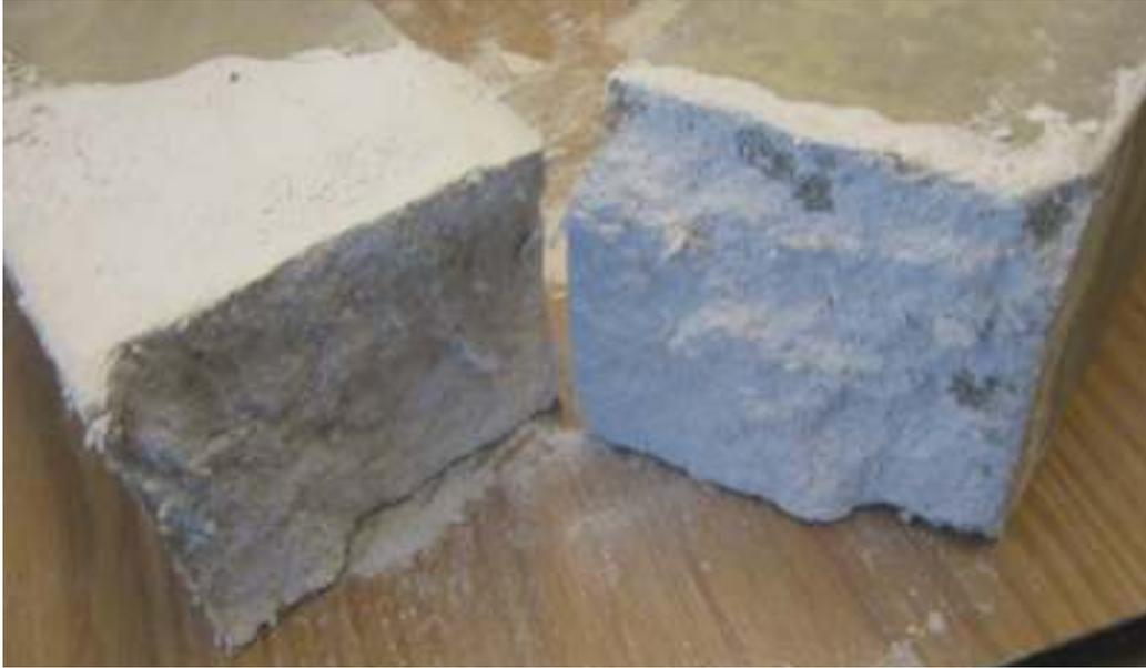
Figure 6.12 Failure of Masonry Unit within the Mortar
