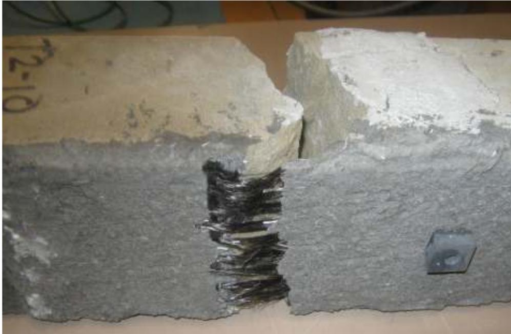
Figure 7.10 Mode of Failure of Composite Sandstone/CTRM Specimen Unit-R-2
