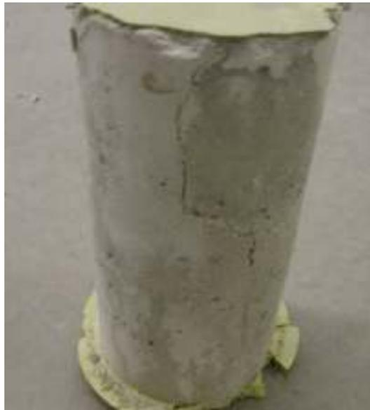
Figure 5.4 Failure of Cylinder for Fibre-reinforced Type S Mortar under Compression
