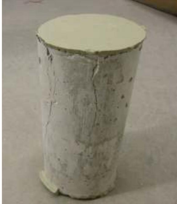
Figure 5.3 Failure of Cylinder for Plain Type S Mortar under Compression
