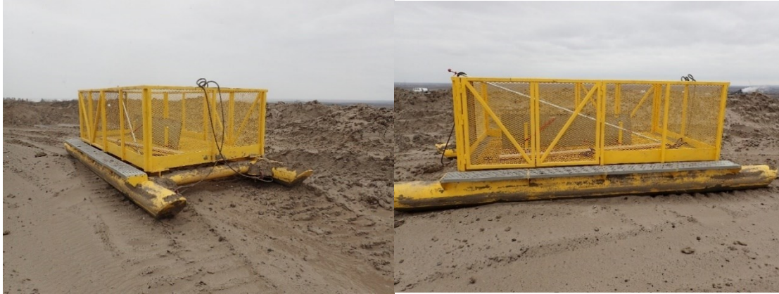
Figure 21. Rescue skids for a tailings discharge area that can be hooked up to a bulldozer.
