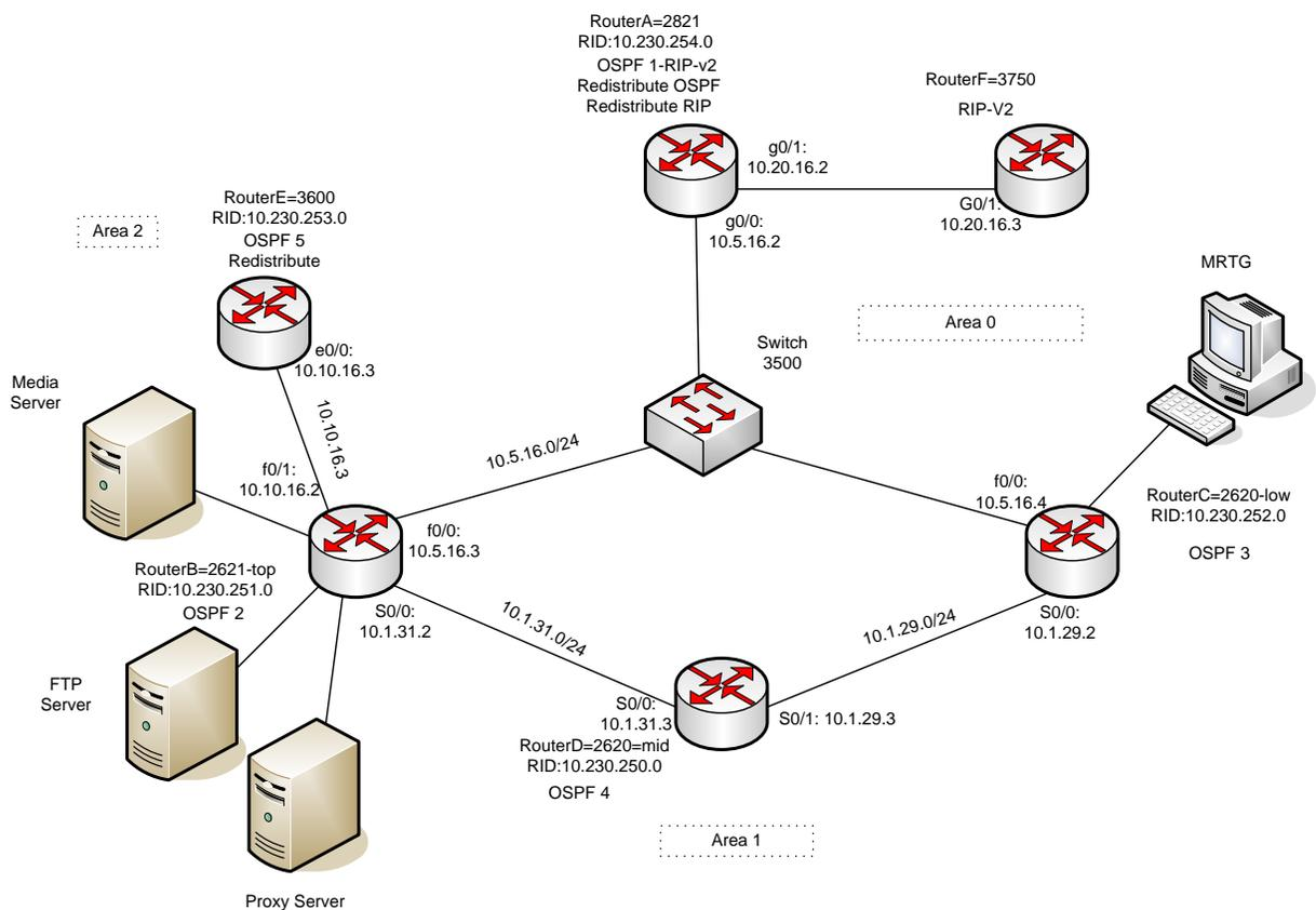
The above fig showing network established in MINT lab for the project. IP addresses are assigned to each router ports, as shown three areas are created and DR and BDR are assigned.
