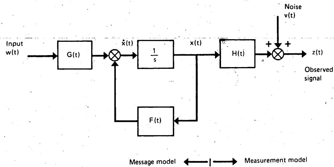
Figure 2.1 Block diagram of the message and measurement models
