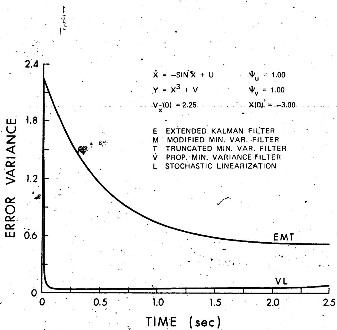
Figure 3.2 The output run of the error-variance for systems with  $\hat{x}(0)=0.0$ ,  $x(0)=-3.0$ ,  $\Psi_u=\Psi_v=1.0$ , and  $V_x=2.25$
