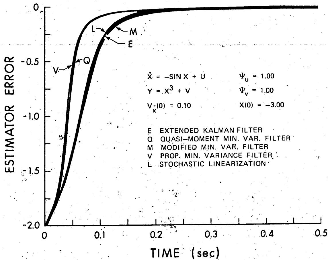
Figure 3.5 The output run of the estimator error for systems
