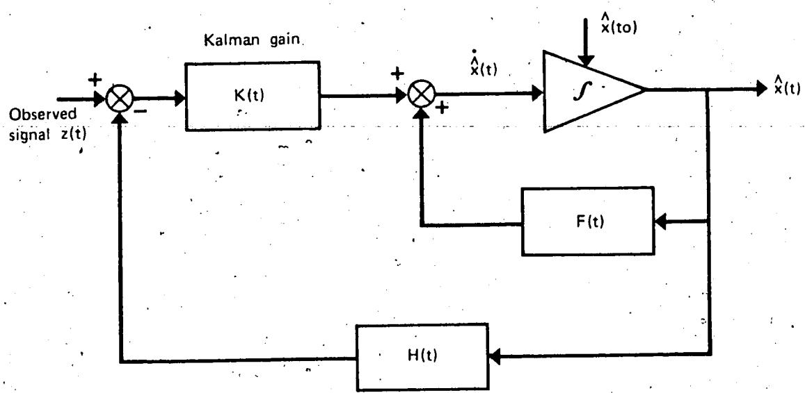
Figure 2.2 Block diagram of the Kalman filter
