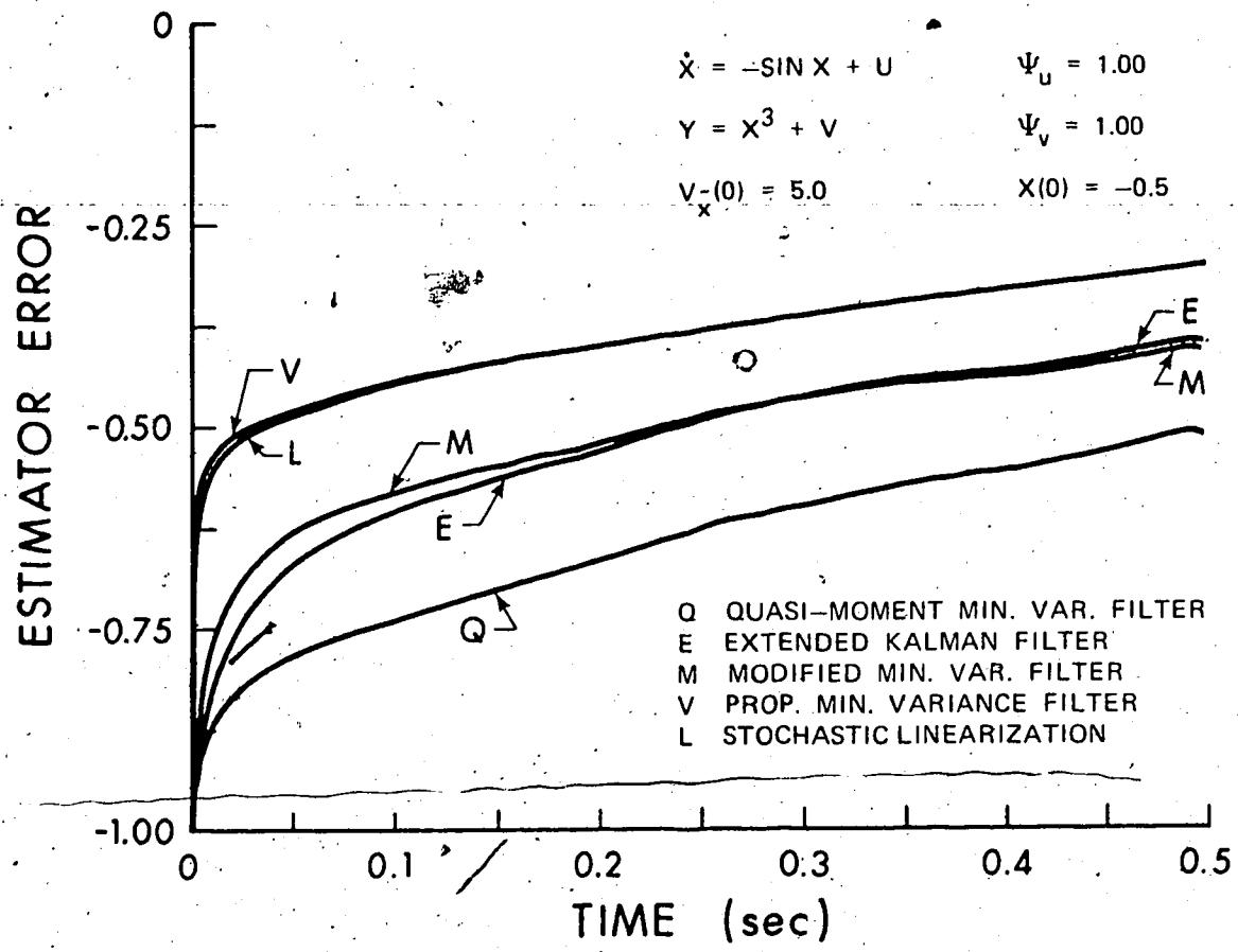
Figure 3.7 The output run of the estimator error for systems
