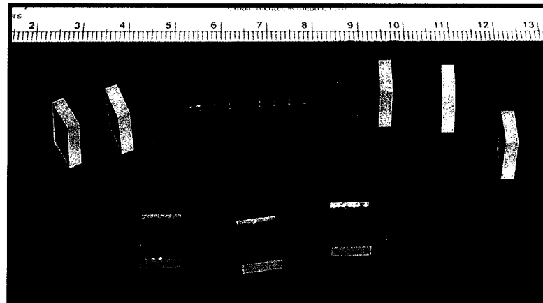
Figure 3.4: Photograph of photodiodes and single CdWO 4 crystals (Courtesy of Dr. Berndt, CancerCare Manitoba, Winnipeg, Manitoba).
