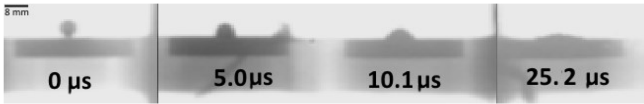
595 Figure 2-11 – Series of flash X-ray images showing the progression of the interaction between the projectile and target. At time 0 \mu\text{s} the projectile has made contact with the target and shows a circular shape, indicating that has not undergone deformation from its initial spherical shape. By 5.0 \mu\text{s} after impact, the projectile is already showing considerable deformation and by 25.2 \mu\text{s} after impact it is nearly flat, demonstrating interface defeat.
