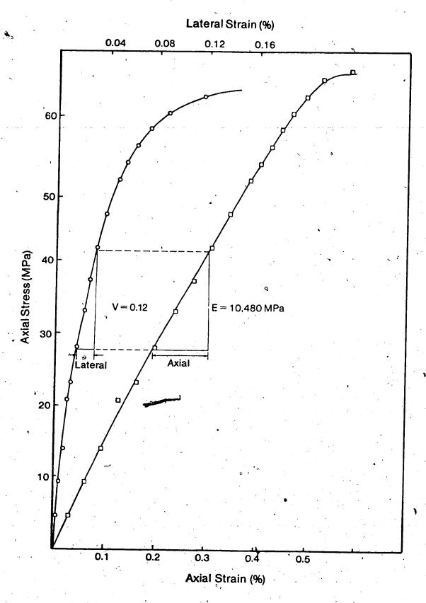
Figure 44a. Axial and Lateral Strains During Uniaxial Compression of Specimen # 98B
