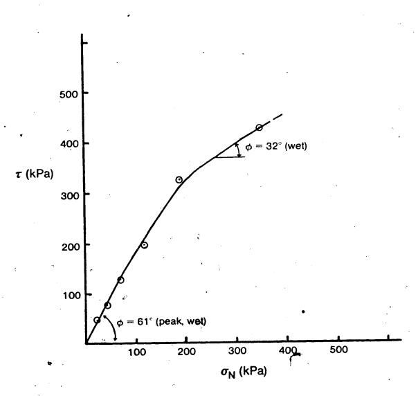
Figure 25a. Shear Strength Versus Normal Stress Along Joint Specimen # 4b.
