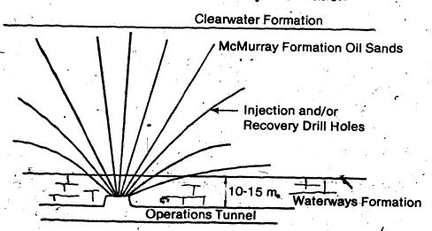
Figure 5 c. d. Diagrams of Proposed Bitumen Recovery Methods
