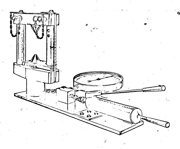
Figure 35. The Point-Load Test Set-Up.
