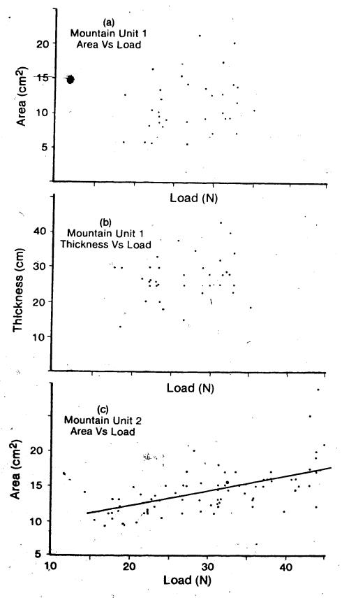
Figure 53. Graphs of Field Point Load Testing
