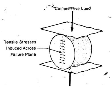
Figure 33. The Brazilian Test Set-Up.
