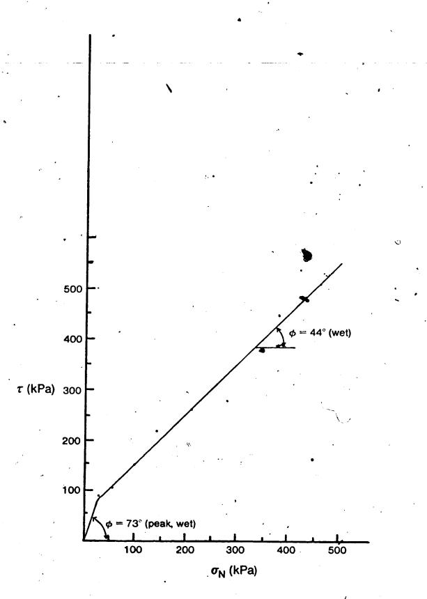
Figure 25b. Shear Strength Versus Normal Stress Along Joint Specimen # 8b.
