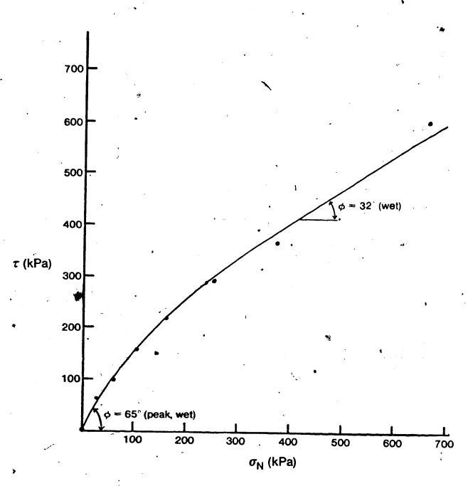
Figure 25c. Shear Strength Versus Normal Stress Along Joint Specimen # 9/10-1.
