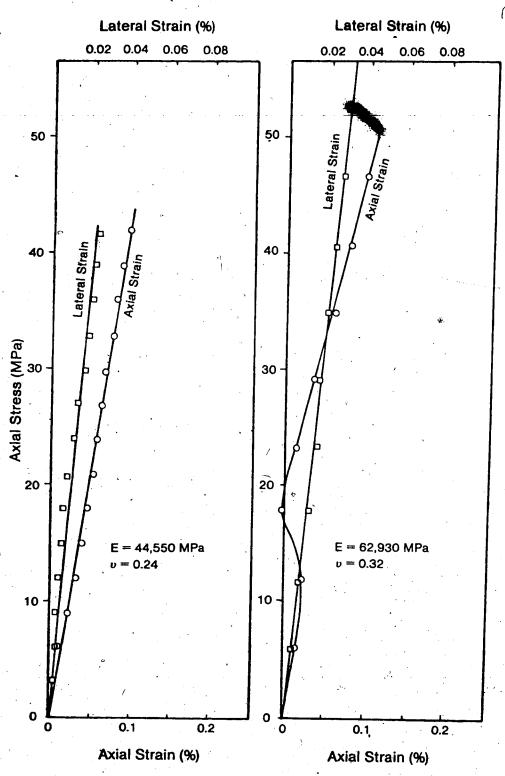
Figure 45. Axial and Lateral Strains in Specimen # 49a (Massive).
