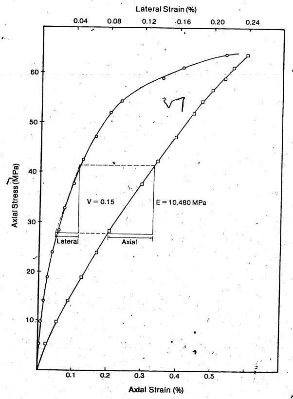
Figure 44b. Axial and Lateral Strains During Uniaxial Compression of Specimen #100f.
