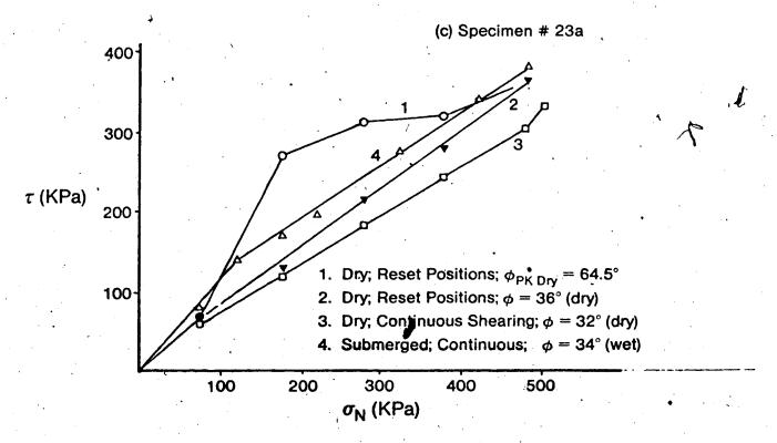
Figure 28. Shear Strength Versus Normal Stress Along Bedding in Specimen # 23a.
