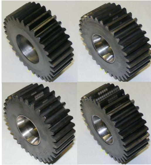
Figure 4-5: View of four artificially pitted planet gears
