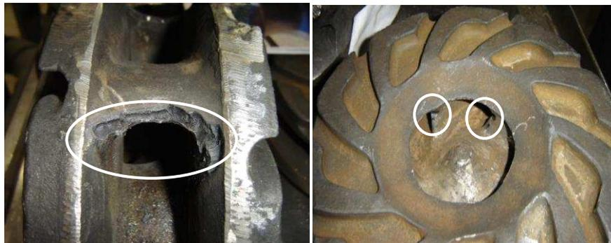
Figure 4-10: Trailing edge damage (left) and leading edge damage (right)
