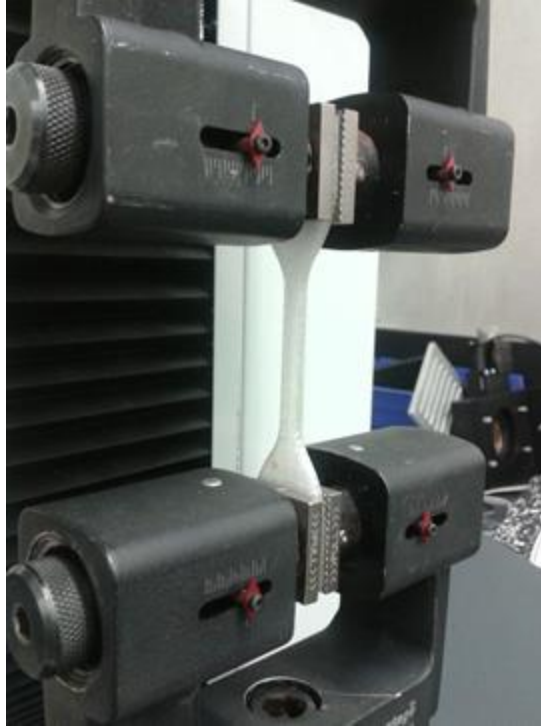
Figure 2: MTS Synergy 400 experimental setup to evaluate test specimen material properties
