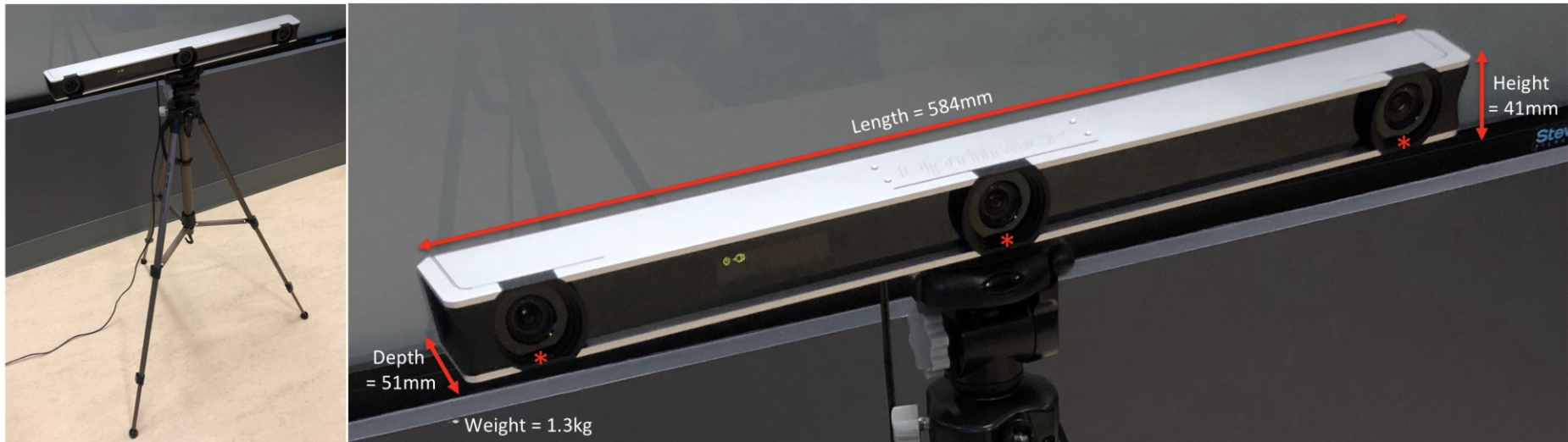
Chapter 2, Figure 2: The optical tracking device containing 3 infrared cameras (+tripod, left; zoomed view, right) used to track transducer and chest marker position in our study (OptiTrack V120:Trio, 6 degrees of freedom, resolution 640x480 x 3, refresh rate 120Hz). The height of the tripod ranged from approximately 120-150cm and was individualized to optimize the line of sight between the cameras and both the transducer and markers. Asterisks correspond to each of the three infrared cameras.
