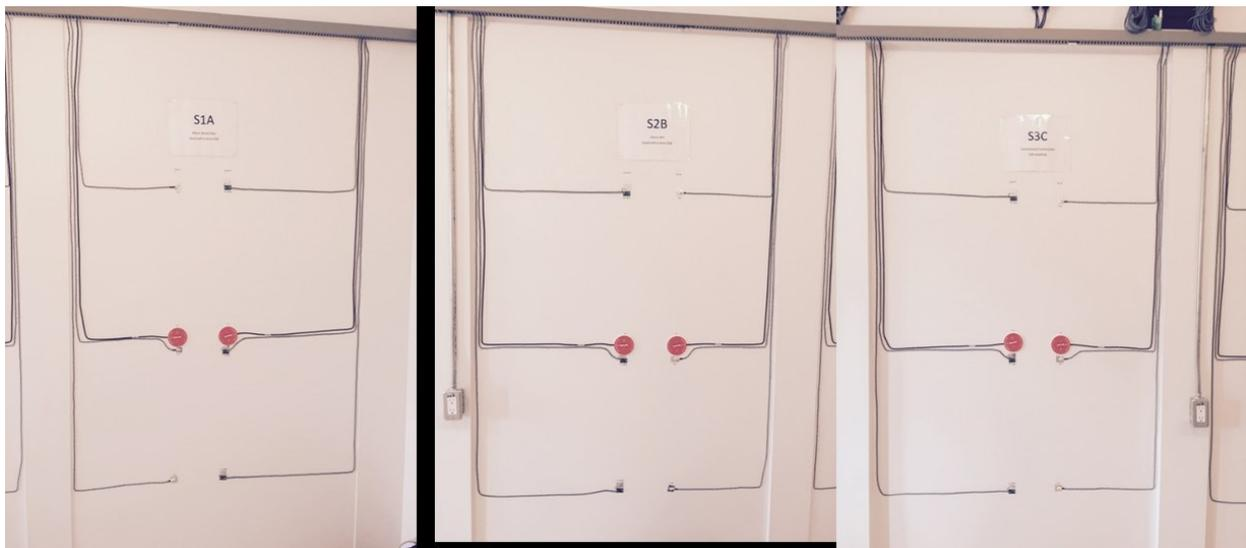
Figure 12: Sample of internal wall of the test huts with sensors applied.
