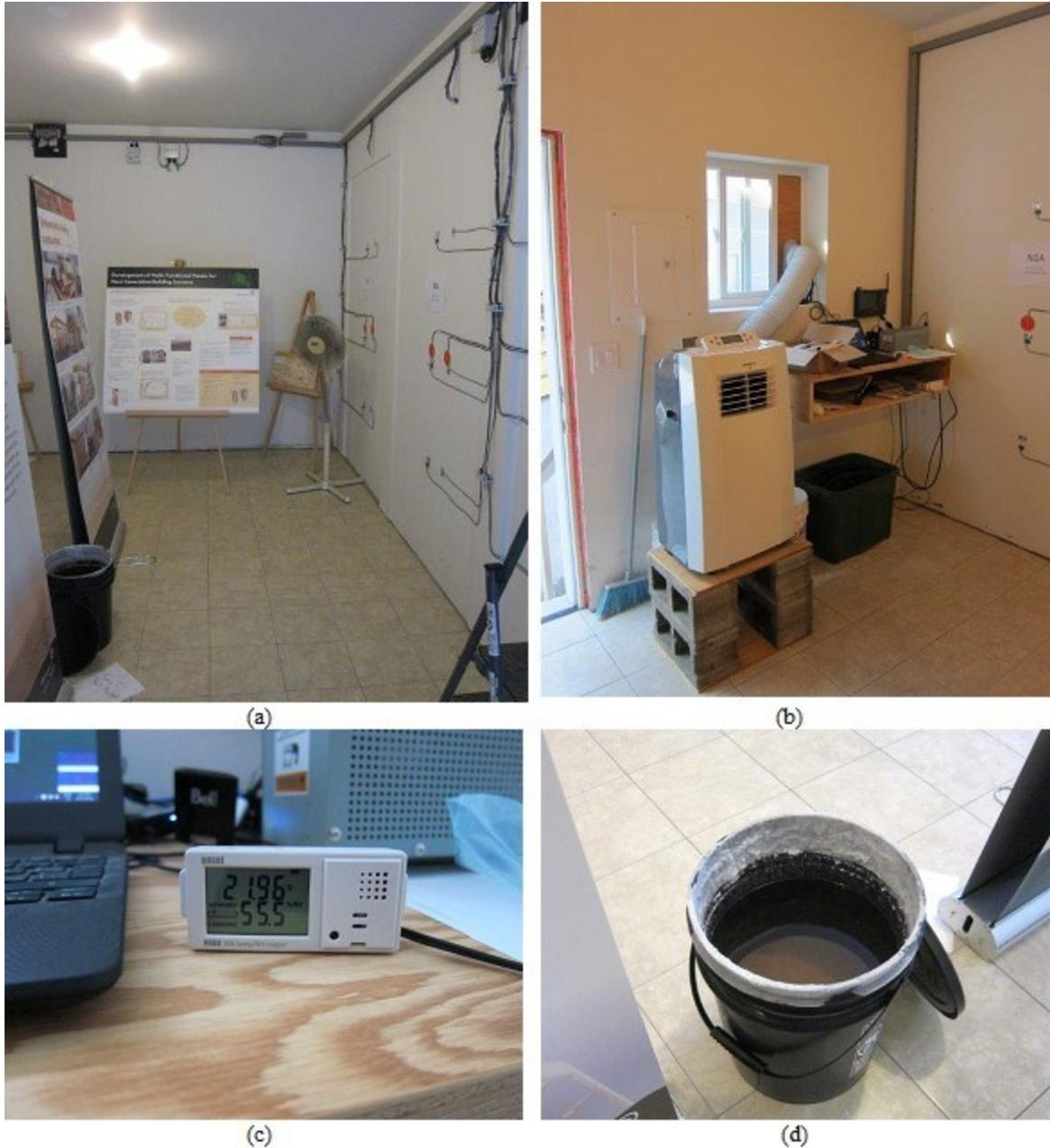
Figure 16: Experimental set up in Vancouver: (a) oscillating fan; (b) air conditioning unit; (c) display with indoor conditions; and (d) NaCl added to water pail.
