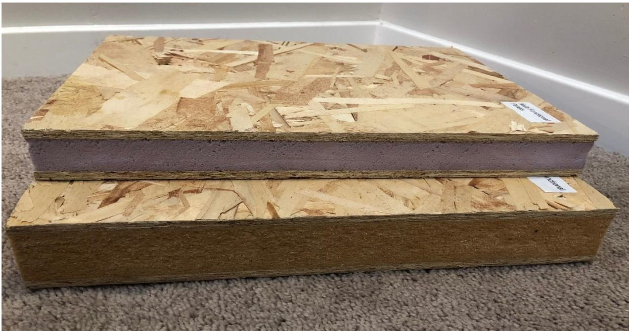
Figure 1: Samples of the multi-functional panel layouts: “Type A” (bottom) and “Type B” (top).
