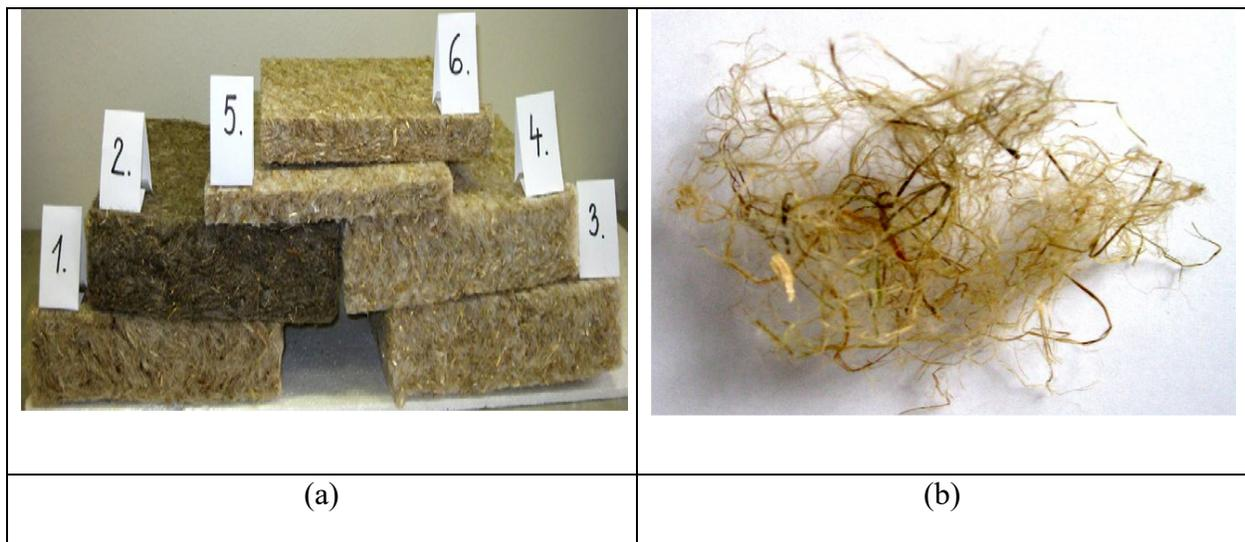
Figure 3: (a) Testing samples and (b) hemp fibres with bicomponent fibres.
