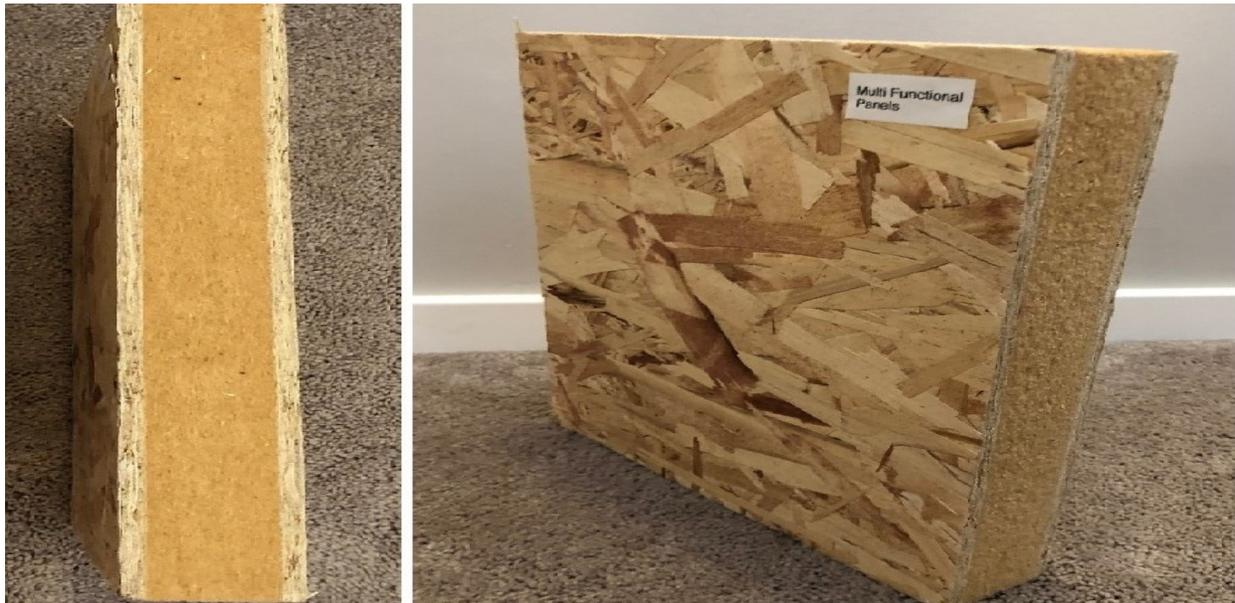
Figure 6: Multi-functional panel “Type A” sample (middle layer of wood fibre and interior/exterior layer of OSB).
