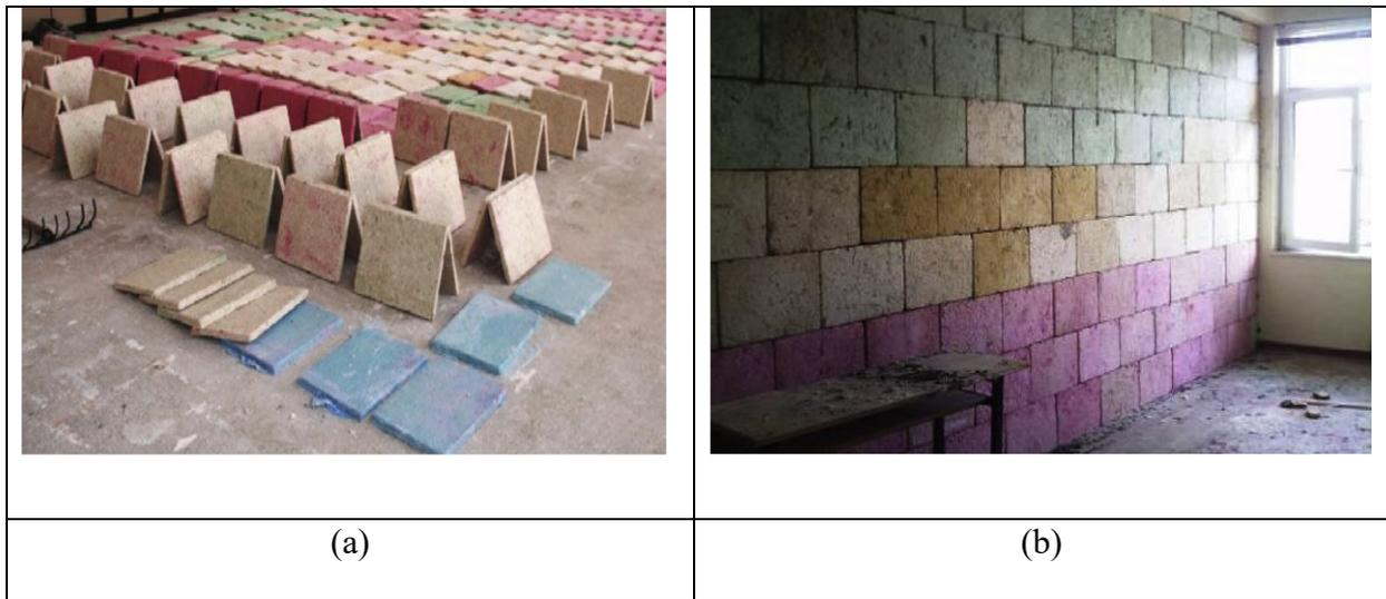
Figure 2: (a) Sample of the materials and (b) application on the interior wall of a commercial building.
