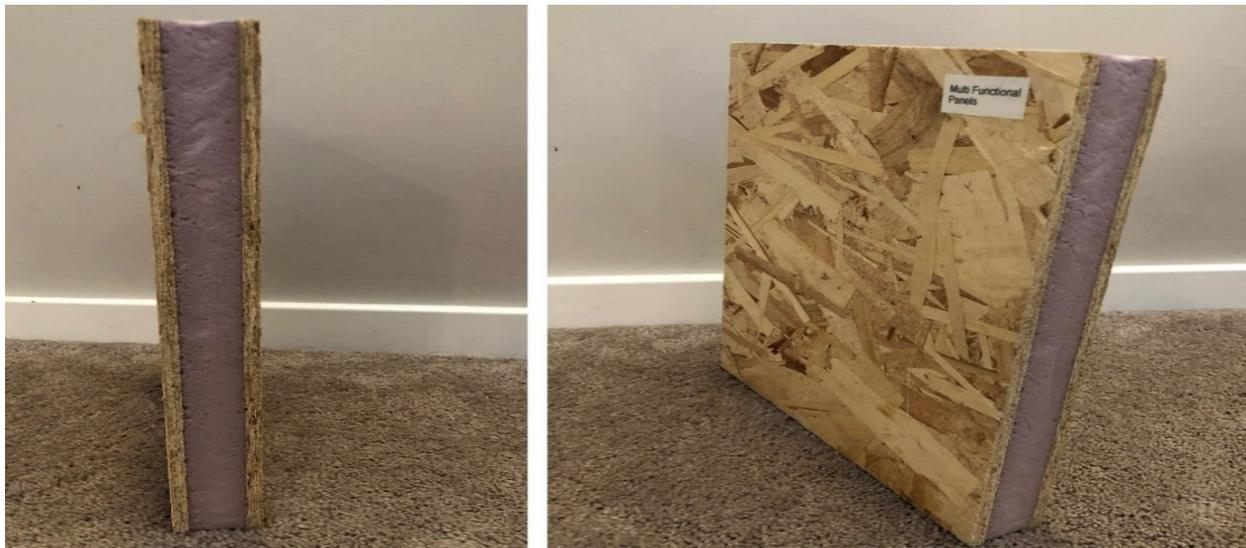
Figure 7: Multi-functional panel “Type B” sample (middle layer of XPS and interior/exterior layer of OSB).
