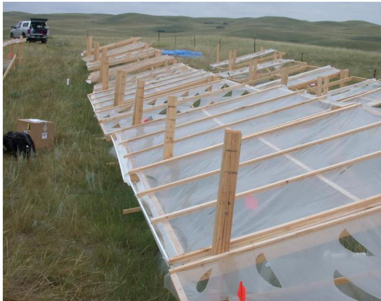
Plate 1-2. Picture showing the set up of transparent rainfall shelter in the study site.
