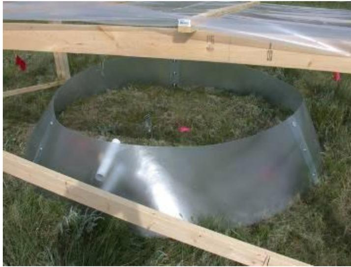
Plate 1-1. Picture showing the set up of open-top chamber in the study site.
