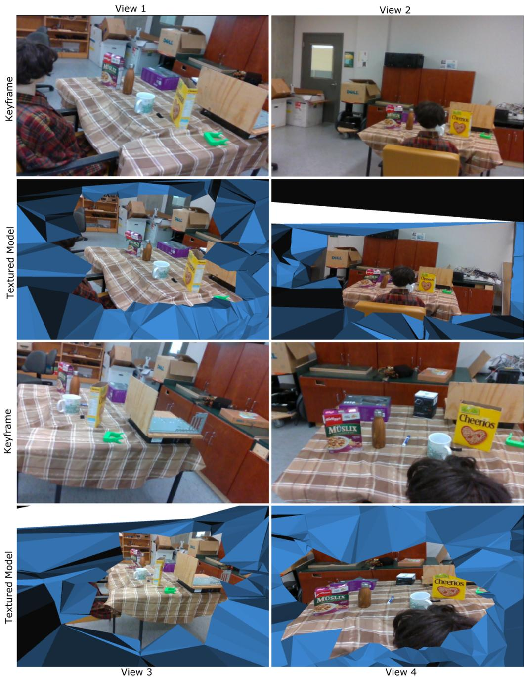
Figure 4.7: Textured Reconstruction of a 3D scene in a real-time setup. Rows 1 and 3 are the reference keyframes and Rows 2 and 4 show the reconstructed model from four different viewpoints
