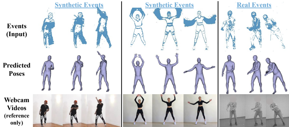
Figure 5.12: Generalization ability of our model, trained solely on the synthetic SynEventHPD dataset and applied to unseen scenarios.
