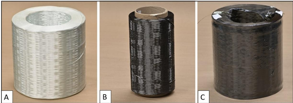
**Figure 3. Roving's of commonly used fibers. (A) glass, (B) carbon, (C) basalt.**
