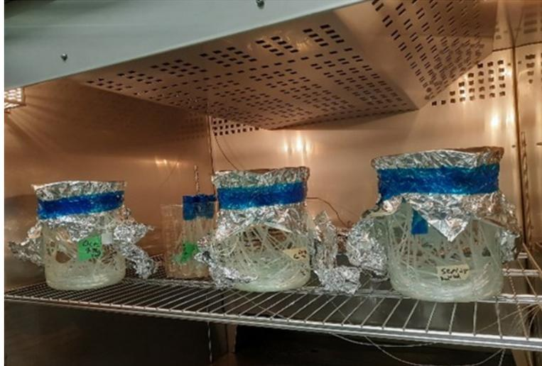
**Figure 8. Aging of fiber samples inside oven.**
