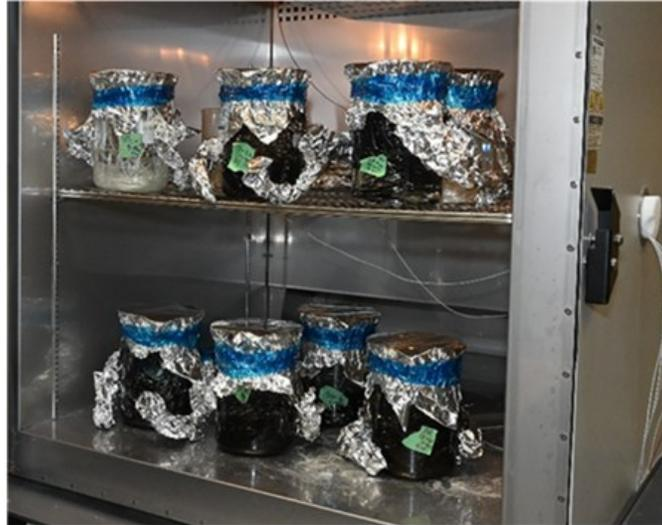
**Figure 17. Aging of samples inside the oven.**
