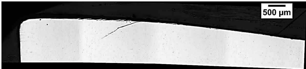
Figure 2.20 Cracks in the mid-gauge region of Rail 10 (Rail 10-TG).
