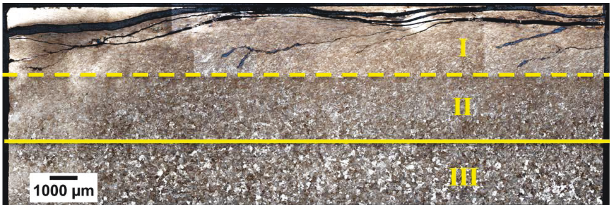
Figure 2.29 (I) Largely deformed, (II) Mildly deformed and (III) Undeformed regions in longitudinal section of the mid-gauge region of Rail 1 (Etched Rail 1-LT).
