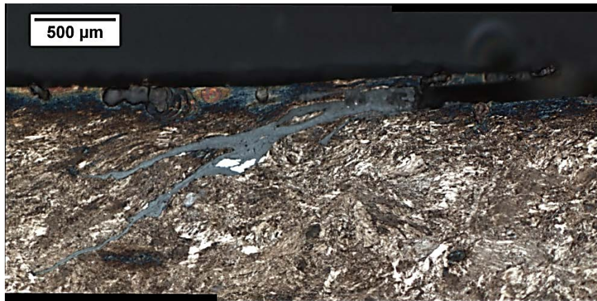
Figure 2.77 Oxidation products inside a crack.
