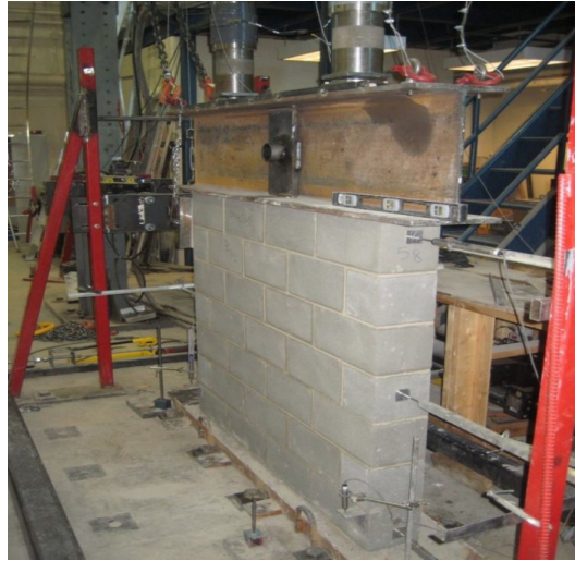
Figure 2.15 – Experimental Test Setup (Oan, 2013)
