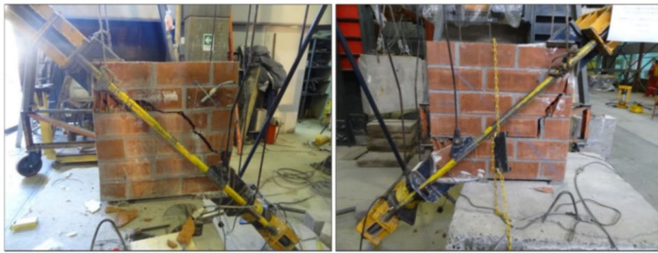
Figure 3.6 – Diagonal Tension Tests (Sandoval and Arnau, 2017)
