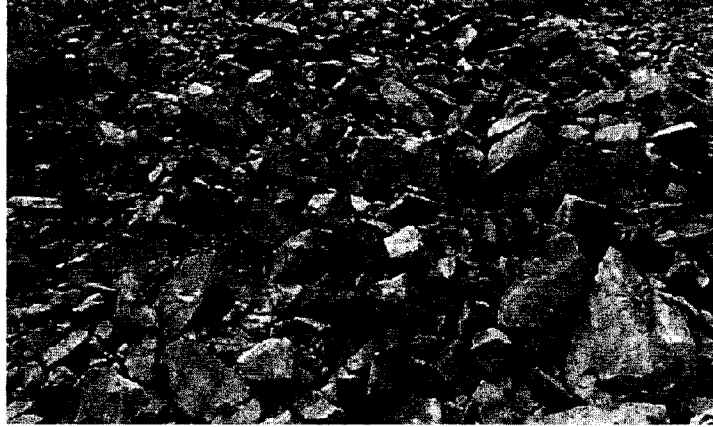
Figure 1.2: An example image 1 of hard rock fragments. The fragments in this image are clearly visible with strong edge definition, and relatively uniform texture and intensity.
