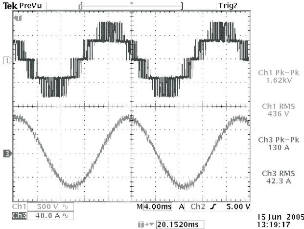
Fig. 7. Oscilloscope trace of voltage  $V_{ab}$  and  $I_a$  (real-time simulation).
