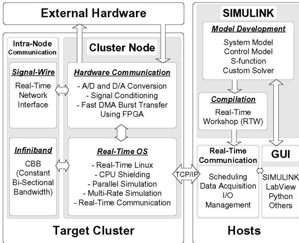
Fig. 3. Functional block diagram of software used in the RTX-Lab simulator.
