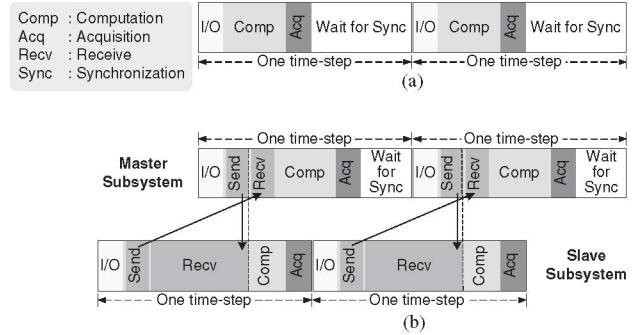
Fig. 4. Time-step anatomy of: (a) single-subsystem case, (b) two-subsystem cases.
