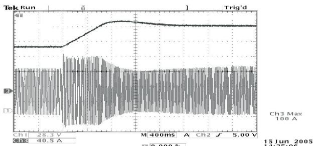
Fig. 10. Oscilloscope trace of transient response of  $\omega_m$  and  $I_a$  (real-time simulation)
