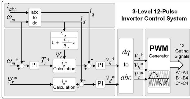
Fig. 6. Control scheme for the variable-speed AC drive.
