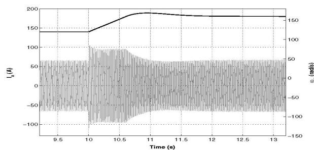
Fig. 11. Transient response of  $\omega_m$  and  $I_a$  (off-line simulation).
