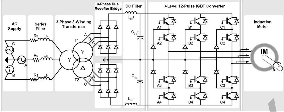
Fig. 5. Electrical system of vector-controlled variable-speed AC drive.
