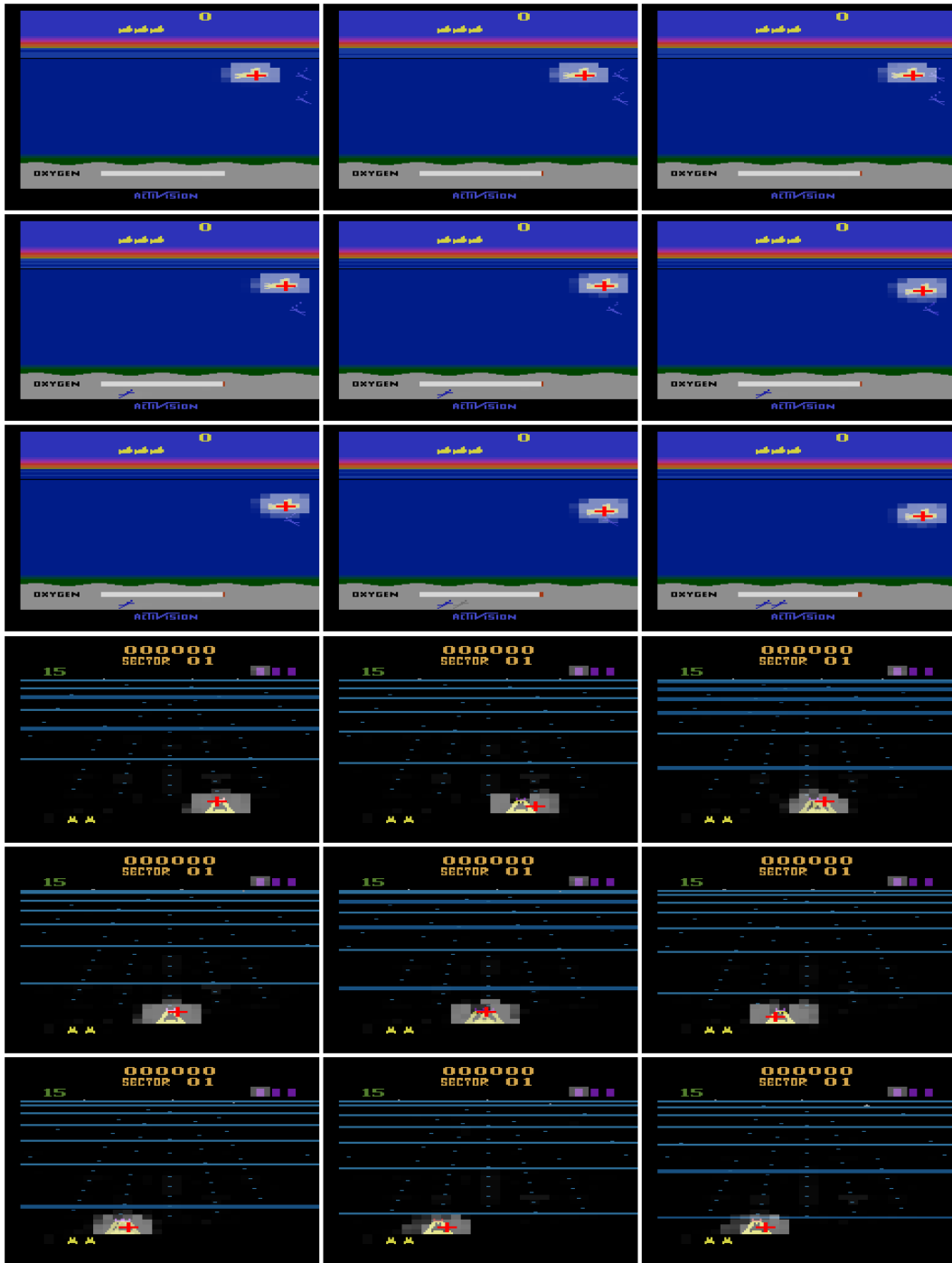
Figure 4.6: Avatar tracking in SEAQUEST and BEAM RIDER. The predicted contingent regions is overlaid in white and the estimated location is indicated by the red crosshairs.
