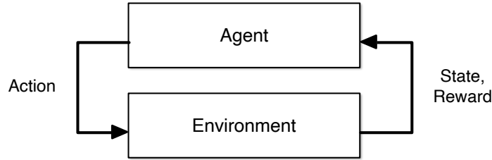
Figure 2.4: A typical representation of a reinforcement learning loop. In the RL setting, an agent learns to maximize the return G by interacting with its environment through actions a while receiving observations of the environmental state s . G is commonly defined as the expected, discounted cumulant of future reward R
