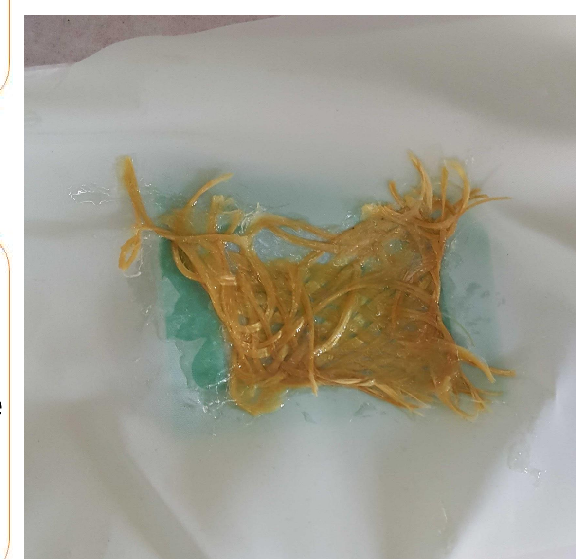
Fig 4: braided composite, sliced and laid flat
