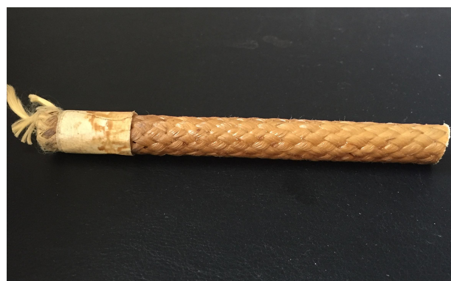
Fig 1: Braided composite tube segment
