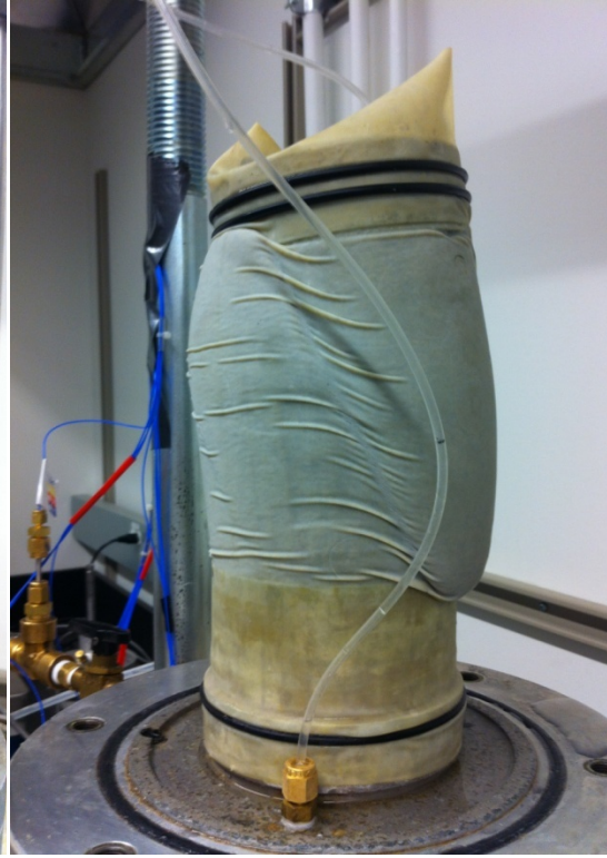
b- Development of visible shear plane in the dense sand specimen
