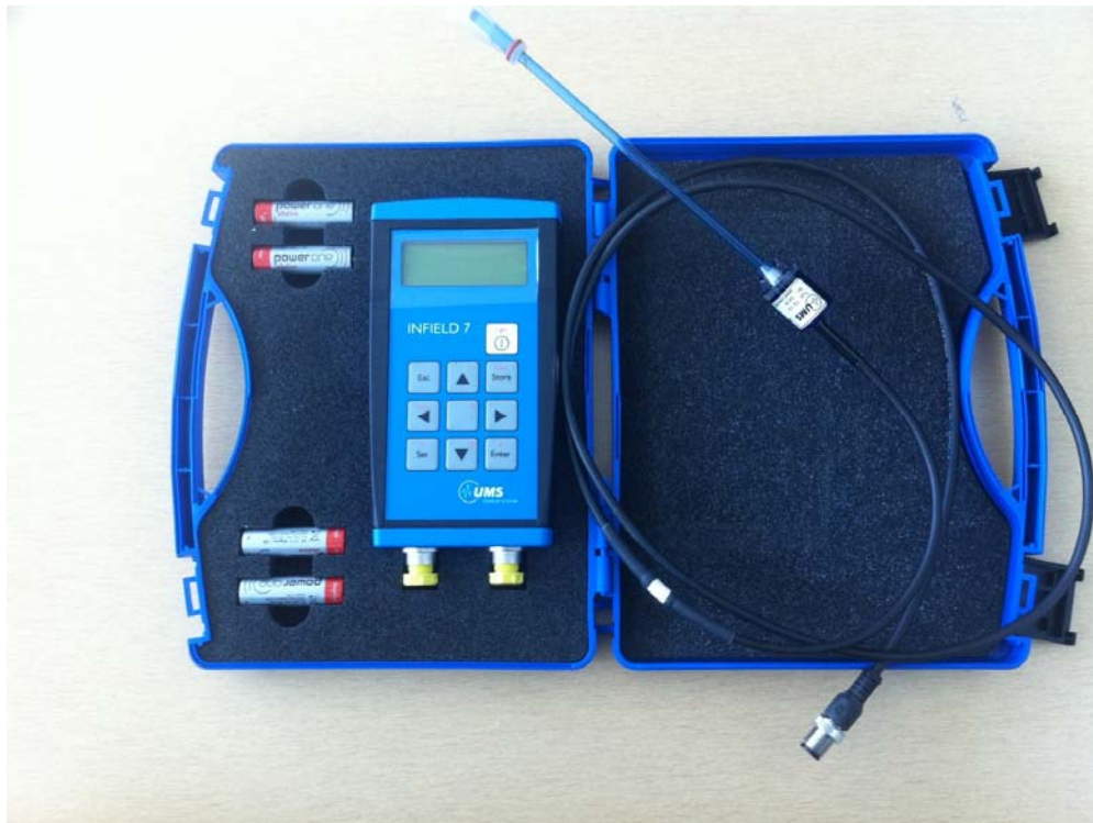
Figure 2-10. Tensiometer model UMS T5-18 and Infield7 datalogger
