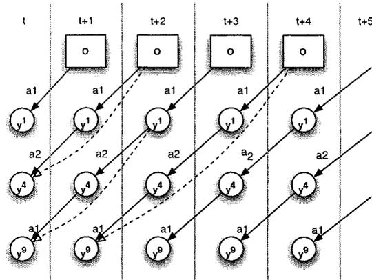
Figure 5.2: Extended target flow diagram for nodes  $\{1,4,9\}$  of question network in Figure 5.1. The links in this diagram show the flow of target values back toward the original predictions. The solid links are the 1-step TD targets for these predictions. The dashed links are a sample of the unrolled multi-step targets. The action-condition labeling have been omitted on the dashed links to reduce clutter.
