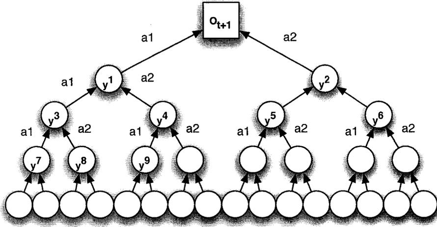
Figure 5.1: Symmetric action-conditional question network. The network forms a symmetric tree, with a branching factor equal to  $|A|$ . This example has depth  $d = 4$ . Some of the labels have been left out of this diagram for clarity, each of these nodes should have a label  $y^i$  and each is conditioned on some action.
