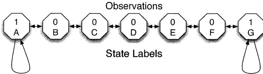
Figure 3.2: Fully observable 7-state stochastic random walk world used in our Markov experiments. The agent is able to observe the label of the state (bottom) and is trying to predict the observation in each step (top).
