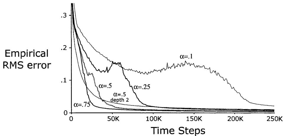
Figure 3.4: Prediction performance on the non-Markov random walk with depth-4 TD networks (and one depth-2 network) with various step-size parameters, averaged over 50 runs and 1000 time-step bins. The “bump” most clearly seen with small step sizes is reliably present and may be due to predictions of different lengths being learned at different times.
