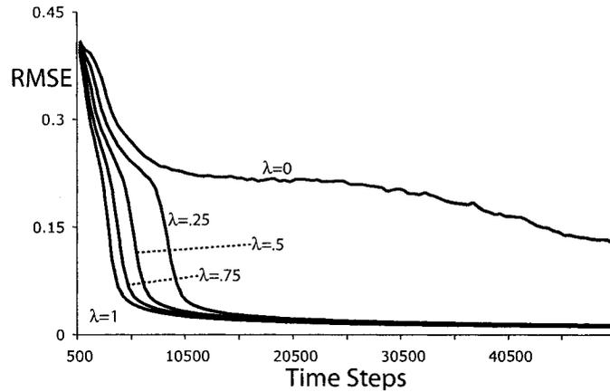
Figure 5.6: Learning curves of our algorithm for various values of  $\lambda$  on the 5-state ring world. This chart represents the average RMSE over all of the nodes in the TD( $\lambda$ ) network. The question network used is of the form seen in Figure 5.1, a full, symmetric, action-conditional question network with depth  $d = 3$ . Each data point in this graph is the average error of the network over 500 time steps. These results are the average of 50 trials.
