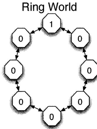
Figure 2.2: An indefinite-memory POMDP problem, the eight-state deterministic ring world. There are two actions in this world, *left* and *right*. *Right* advances in clockwise rotation while *left* advances in counter-clockwise rotation. Prediction methods using a finite length history will lose localization after some number of transitions back and forth between the states that emit observation 0.
