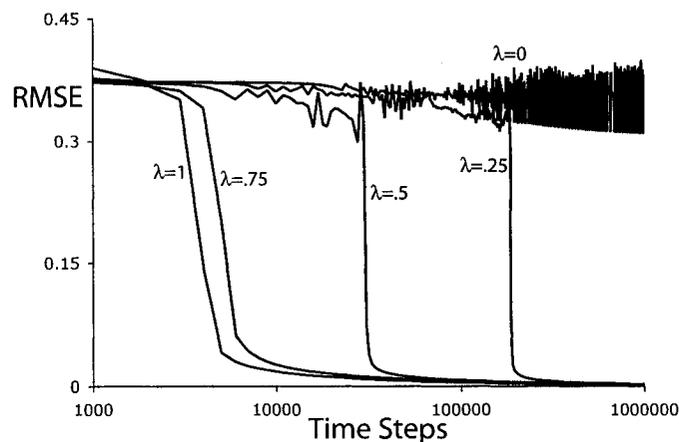
Figure 5.4: Learning curves of our learning algorithm for various values of  $\lambda$  on the 6-state cycle world. This chart represents the average RMSE over all of the nodes in the TD( $\lambda$ ) network as the amount of data is increased. Each data point in this graph is the average error of the network over 500 time steps. Note that the x-axis (amount of data) is an exponential scale. The cycle world is completely deterministic, so these results are for a single training run.
