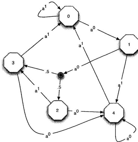
Figure 2.1: Graphical representation of a simple MDP with 5 states and 2 actions. The .5 links coming from state 1 correspond to a stochastic transition; taking action  $a^0$  in state 1 can lead to either state 2 or state 3. The observation matrix for this MDP is shown in Table 2.2.
