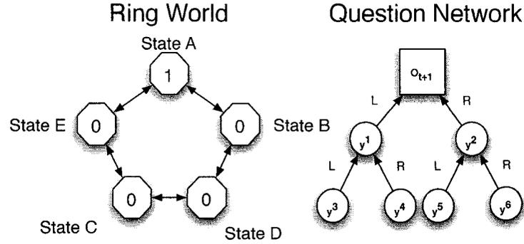
Figure 4.4: An indefinite-memory problem, the five-state deterministic ring world and an example question network of depth 2. There are two actions in this world, *left* or simply *L* and *right* *R*. *right* advances in clockwise rotation while *left* advances in counter-clockwise rotation. Prediction methods using a finite length history will lose localization after some number of transitions back and forth between the states that emit observation 0.
