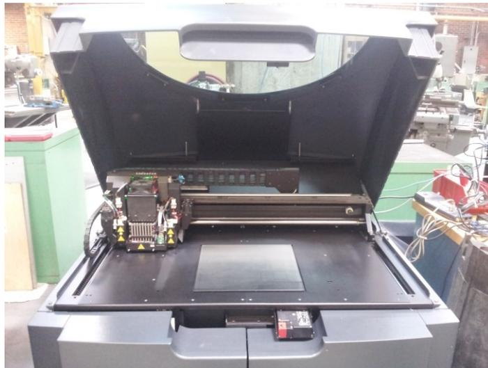
Figure 4-2: Objet Eden350V (Stratasys) that prints UV-curable resin. It is located at Mechanical Engineering department, University of Alberta.
