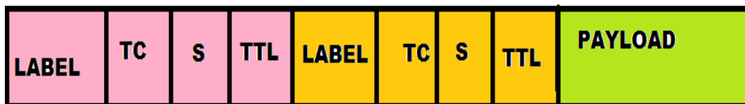
FIGURE 2 MPLS header stack
