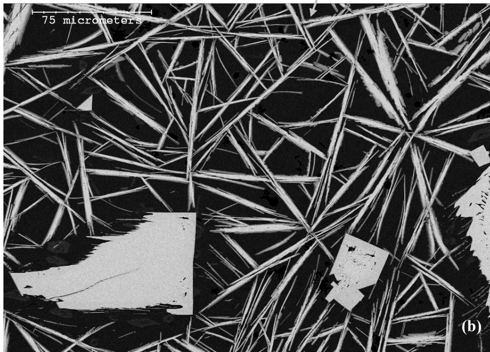
Figure 4.61: BSE image of surface of multiple pass coating, showing acicular secondary carbides at the surface (a) and dissolution of primary WC particles with acicular secondary phase (b)
