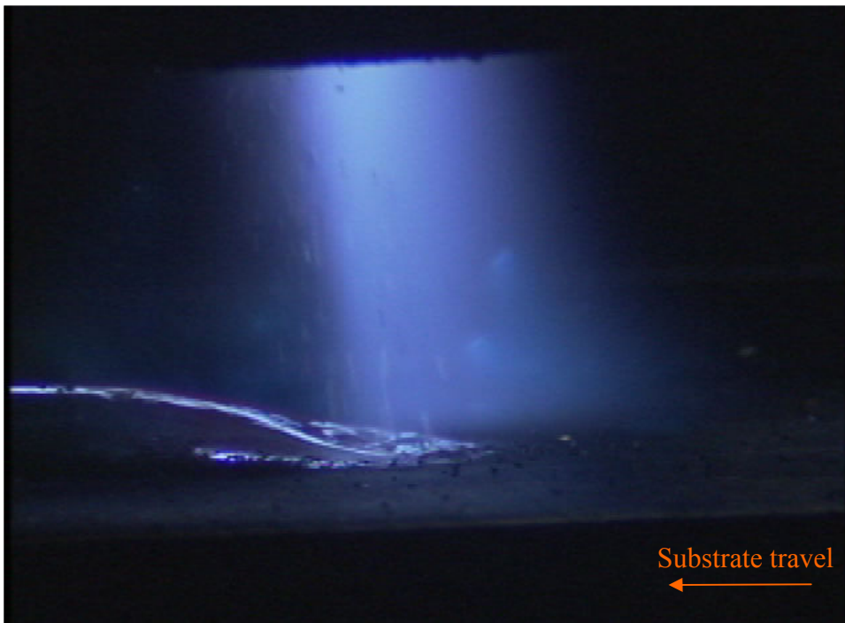
Figure 4.43: Image of plasma arc with NiCrBSi +WC powder addition, and increased current.
