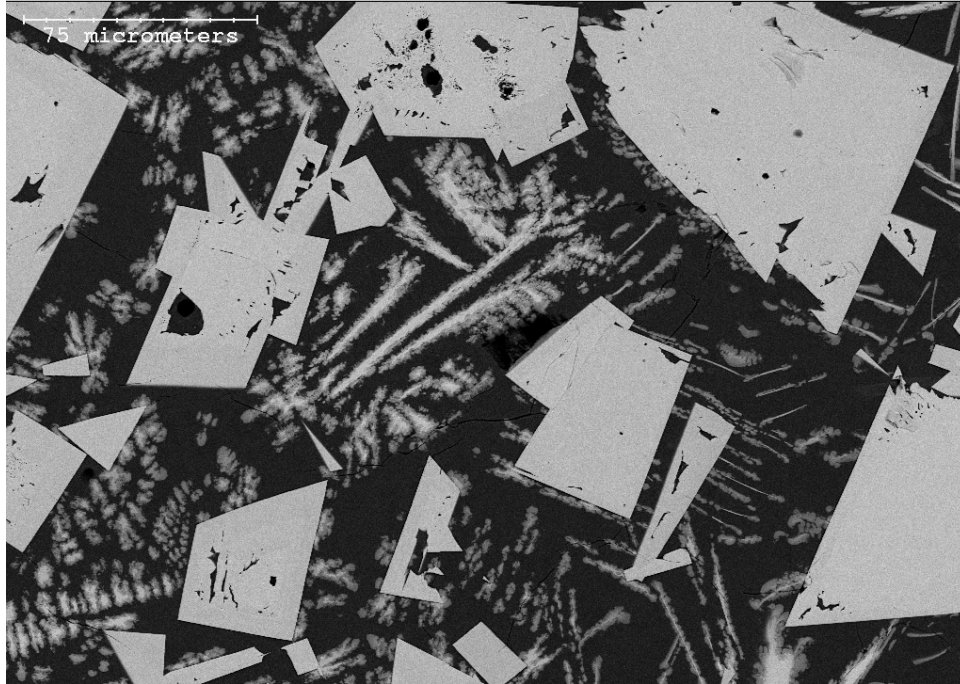
Figure 4.63: BSE image of change in morphology of secondary phase from acicular on surface to dendritic surrounding WC particles further into the matrix
