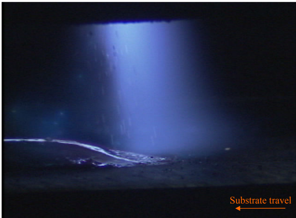
Figure 4.41: Image of plasma arc with NiCrBSi +WC powder addition, under standard conditions.
