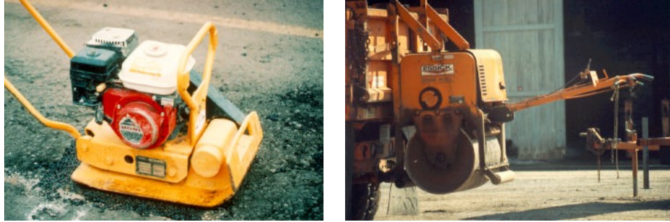
(ii) Compaction of patching material
