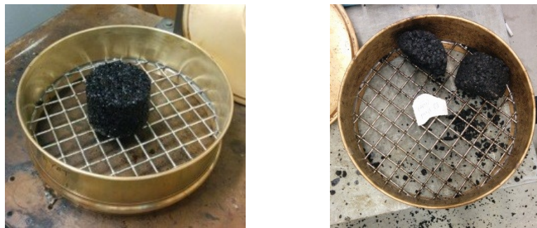
(a) Sample on sieve before testing (b) Retained material after testing
