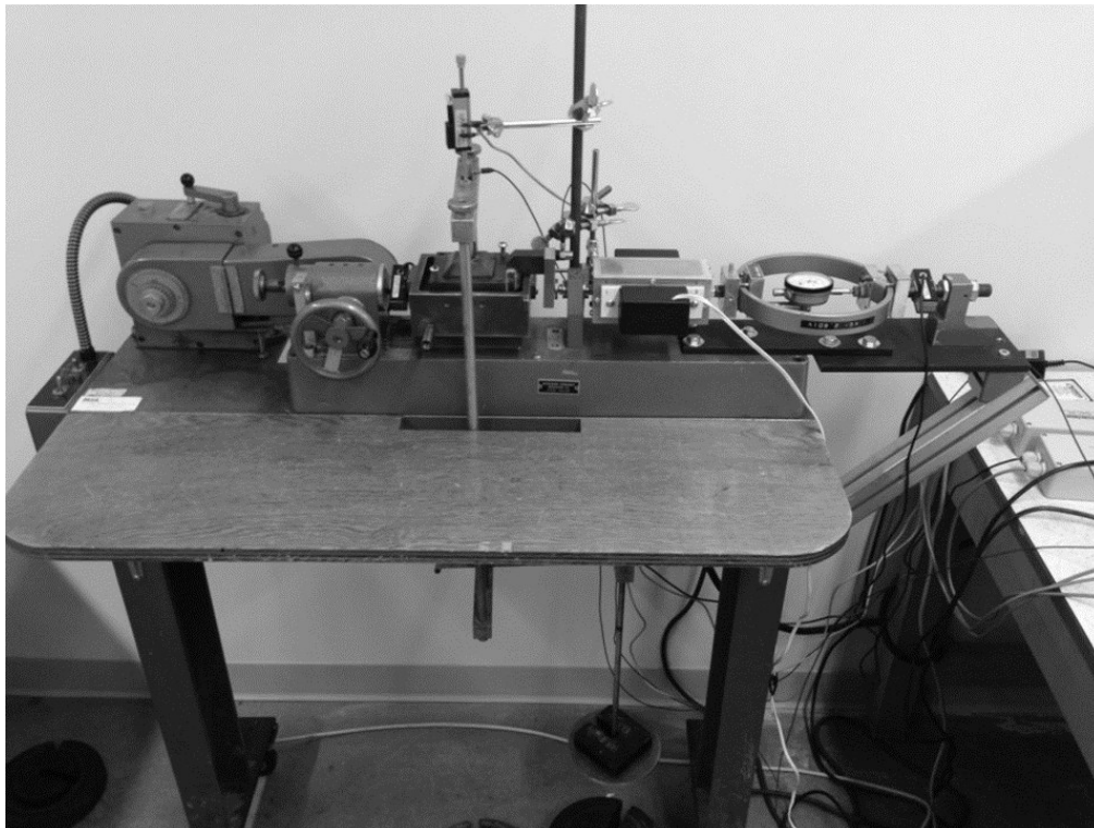
Figure 3.4 Prototype of the strain controlling vibrating direct shear apparatus
