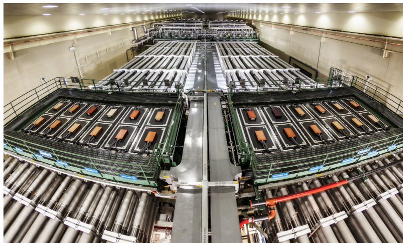
Figure 1.3: Shows one of the two laser bays at the National Ignition Facility. These bays contain 96 each and are 122 meters (400 feet) long. This image was taken from the photo gallery page of the Lawrence Livermore National Laboratory National Ignition Facility and Photon Science website: lasers.llnl.gov/media/photo-gallery .
