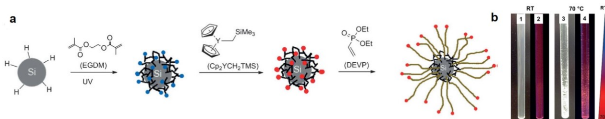
Figure 1-15. a) Schematic of SI-GTP-mediated synthesis of SiNC-g-PEGDM-g-PDEVF HFM, and b) photographs demonstrating the PL and thermoresponsive properties of the HFM; 1) and 2) show a dispersion of HFM in water at room temperature under ambient and UV light, respectively; 3) and 4) are the same dispersions after heating at 70 °C. Reproduced and adapted with permission from Kehrle et al. 182 Copyright 2014, WILEY-VCH.
