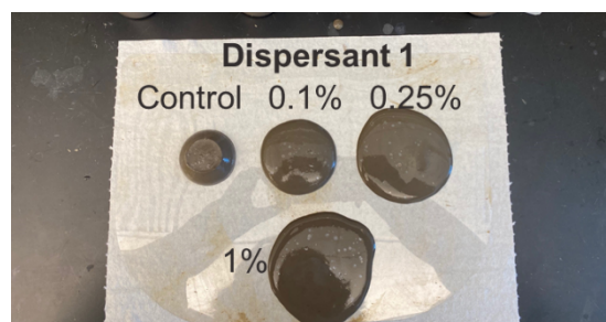
Figure 3. Flowability using different dispersant concentrations (0.1, 0.25 & 1%) vs control.
