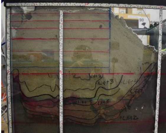
Figure 4: Lift 9 Cap, CST Target Height Traces, and CFFT-CST Interface Traces at Wall
