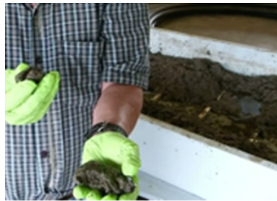
Figure 5. Slurry squeeze by hand to give a consolidate material with a solids content of about 75 wt.%
