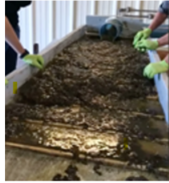
Figure 4. Slurry emerging from the pipes on a flume to give simple gravity dewatering
