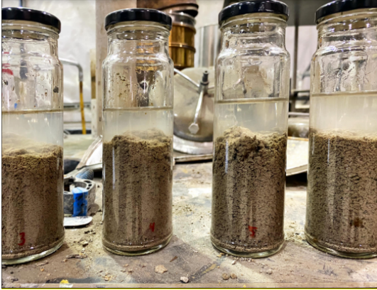
Figure 6. FFT treated with TNS™ solution before centrifugation
