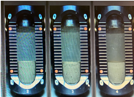
Figure 7. Treated FFT samples during centrifugation / consolidation process
