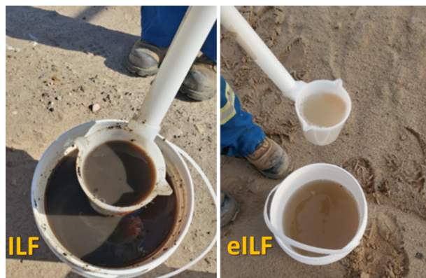
Figure 4. Release water samples collected from the ILF and eILF cells during deposition.
