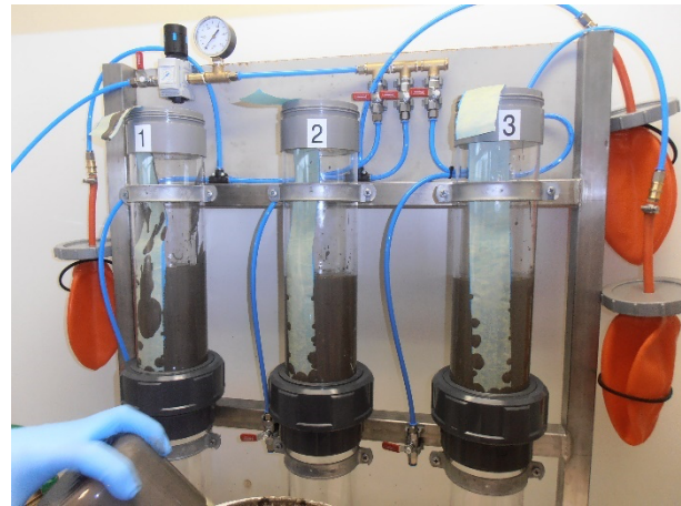
Figure 3. Preparation of the MFT test on Filter conform the methods described in REF
