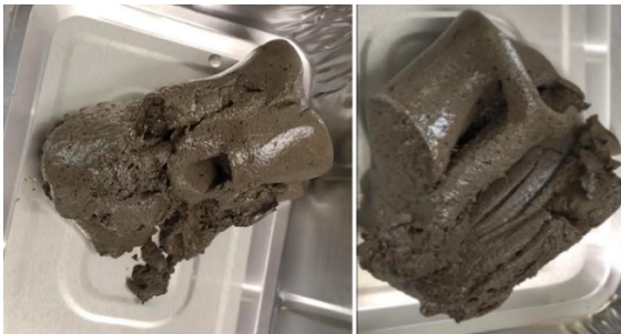
Figure 8. Centrifuge Cake sample for FFT samples treated with TNS™ Technology
