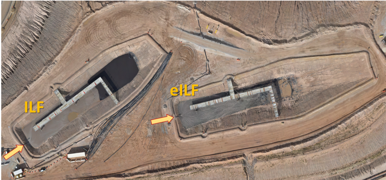
Figure 3 - Aerial Photo of the two test cells (six days after completion of the pour). The arrows show the position of discharge outlet at each cell.
