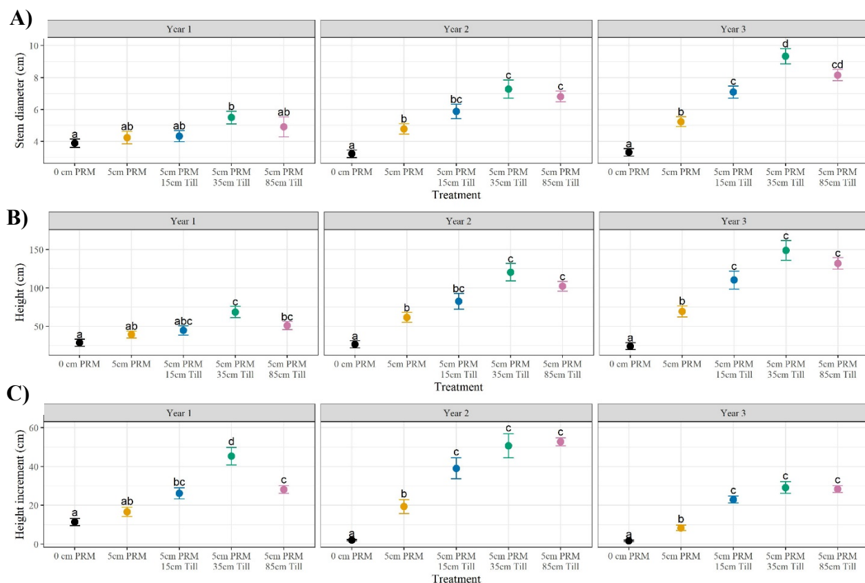
Figure 7. Mean stem diameter (A), height (B), and height growth increment (C) of Salix bebbiana at the end of each year per treatment; 0 cm peat reclamation material (PRM) (black), 5 cm PRM (yellow), 5 cm PRM / 15 cm till (blue), 5 cm PRM / 35 cm till (green), and 5 cm PRM / 85 cm till (pink). Error bars represent standard error of the mean. Differing letters between means indicate a significant difference ( P < 0.05 ).
