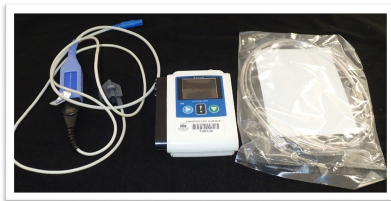
Figure 2.2: Front (left) and top (right) views of a level 4 portable sleep monitor (Embletta MPR, Natus Neurology, Middleton, USA). This particular device has channels to record airflow via nasal cannula, pulse oximetry, and a microphone.
