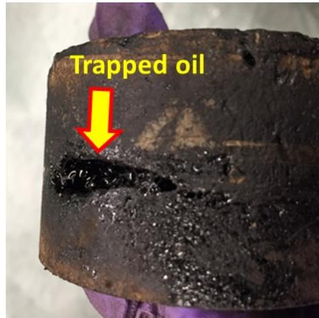
**Figure 5-23. Trapped oil, after experiment with distillate oil at 90°C.**
