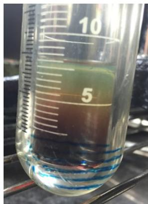
**Figure 5-16.** Fluids produced during experiment performed at 35°C. Solvent injected in liquid form.
