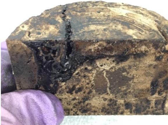
**Figure 5-22. Core after injecting heptane at 73°C showing zones that apparently were not saturated with heavy oil.**
