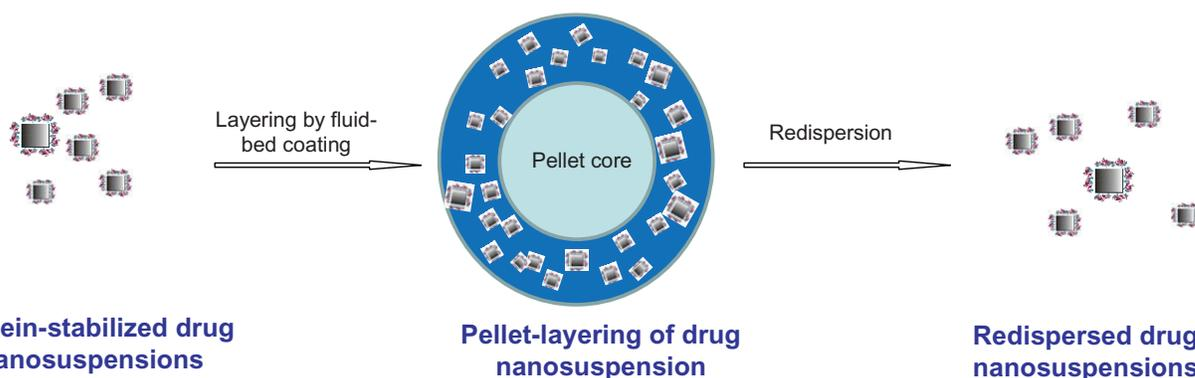
**Figure 1** Schematic representation of the formation of pellets coated by nanosuspensions containing indomethacin.
