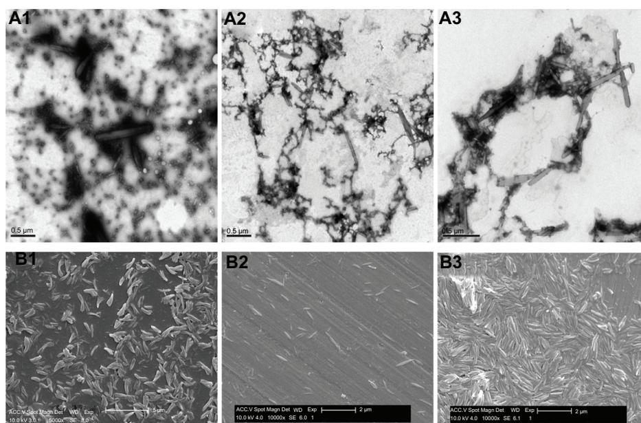
**Figure 2** Transmission (A1–3) and scanning (B1–3) electron micrographs of nanosuspensions stabilized by soybean protein isolate, whey protein isolate, and  $\beta$ -lactoglobulin (from left to right).
