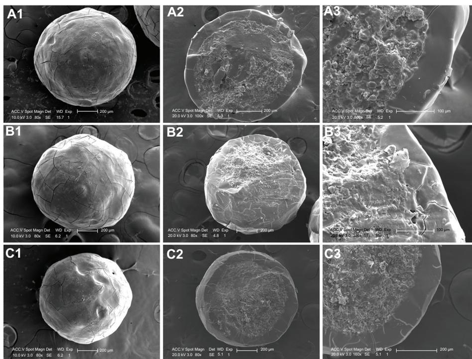
**Figure 3** Scanning electron micrographs of the surface and cross-section of pellets layered by nanosuspensions stabilized by soybean protein isolate (**A1–3**), whey protein isolate (**B1–3**), and  $\beta$ -lactoglobulin (**C1–3**).
