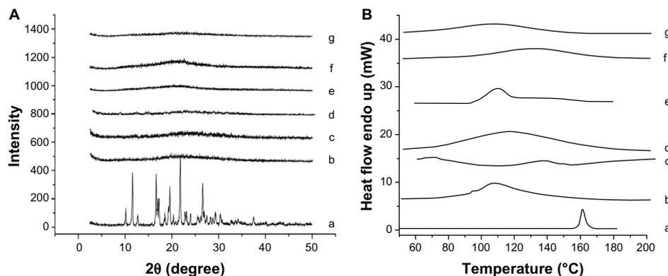
**Figure 6** Powder x-ray diffractograms (A) and differential scanning calorimetry thermograms (B) from bottom to top: raw crystals, freeze-dried powder from nanosuspensions stabilized by soybean protein isolate, whey protein isolate, or  $\beta$ -lactoglobulin, and pellet powder from nanosuspensions stabilized by soybean protein isolate, whey protein isolate, or  $\beta$ -lactoglobulin.
